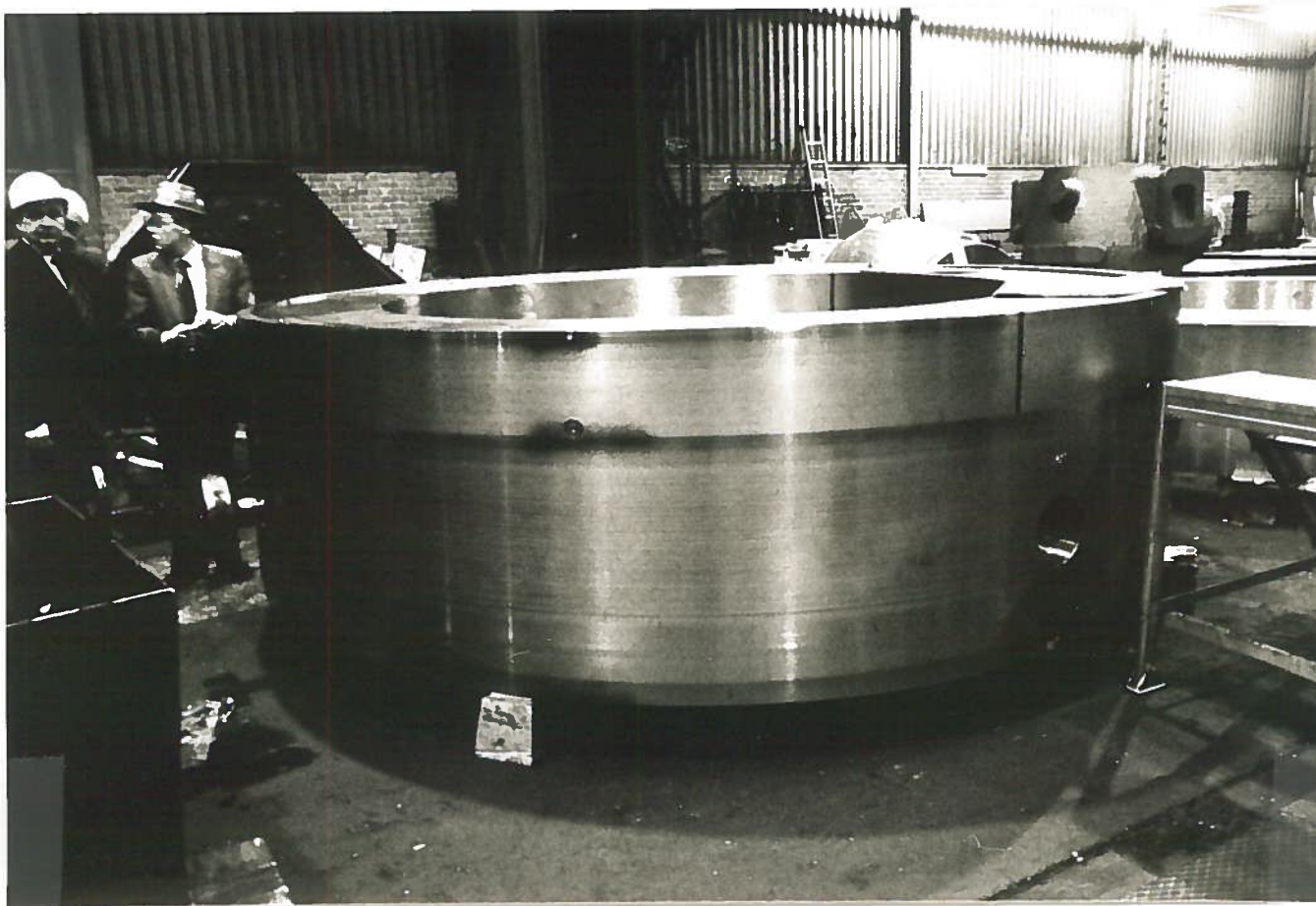
FIG. 30 - View of the lower and central rings after final machining.
