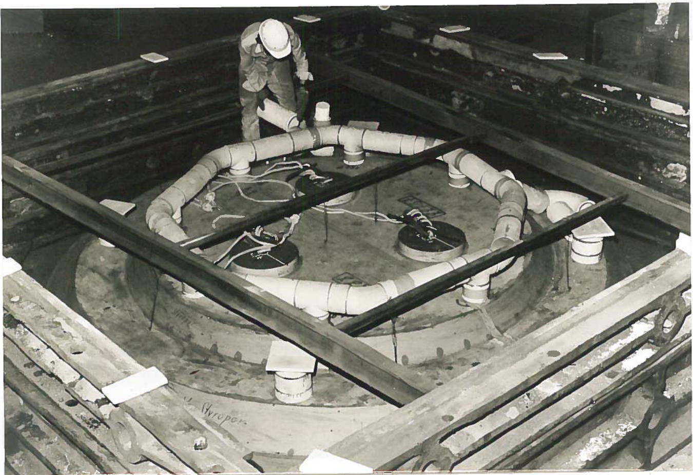
FIG. 19 - Styropore pattern for the casting of the pole caps.
