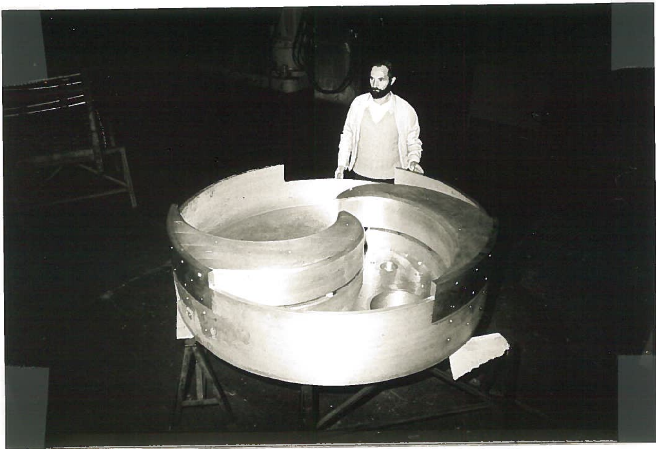
FIG. 48 - View of the aluminum full scale prototype of two sectors, the valley in between and the relevant plate.
