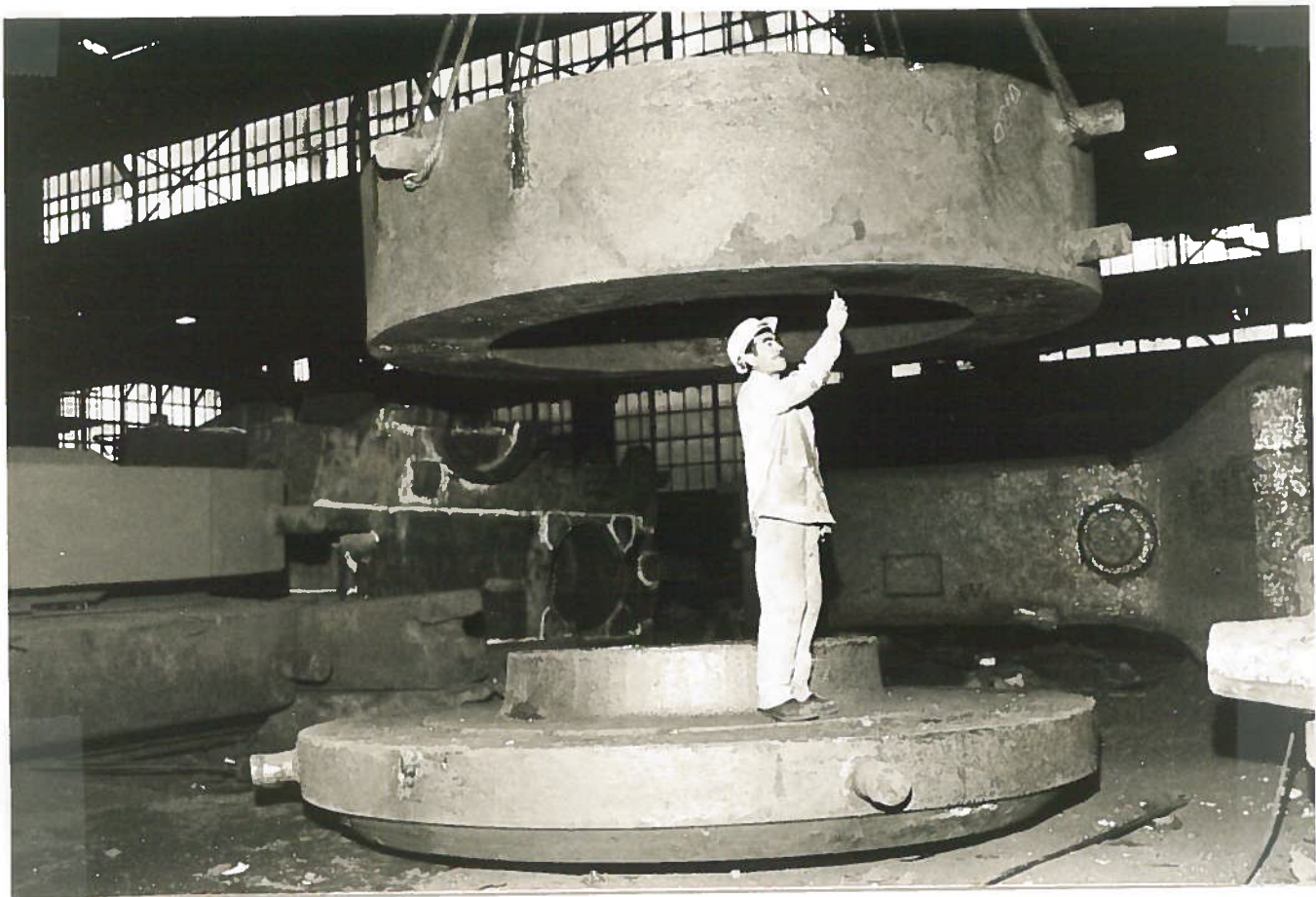
FIG. 21 - View of the lower pole cap and lower ring after casting.
