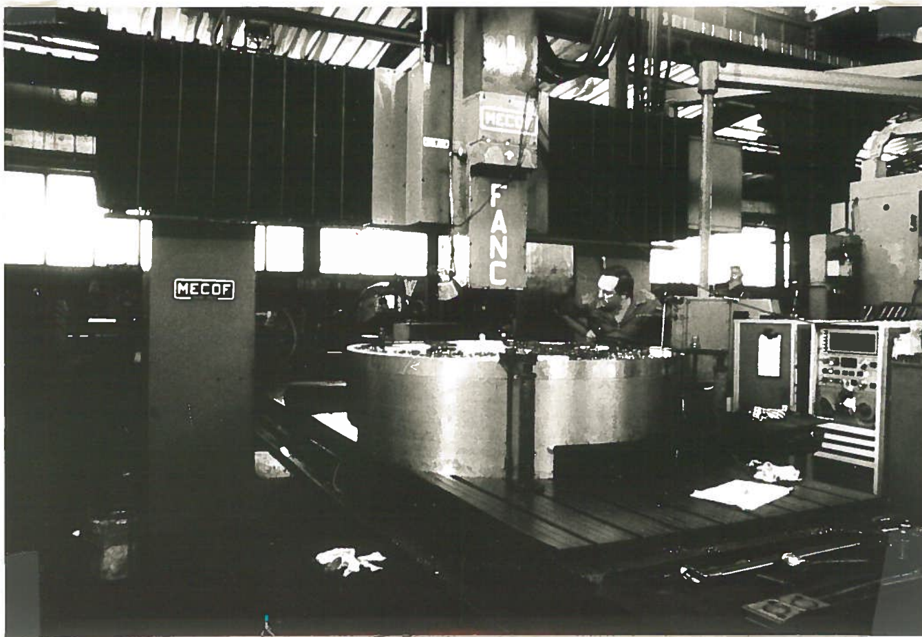
FIG. 66 - View of one pole plate and ring during machining of the holes for the assembly of the lower sectors.
