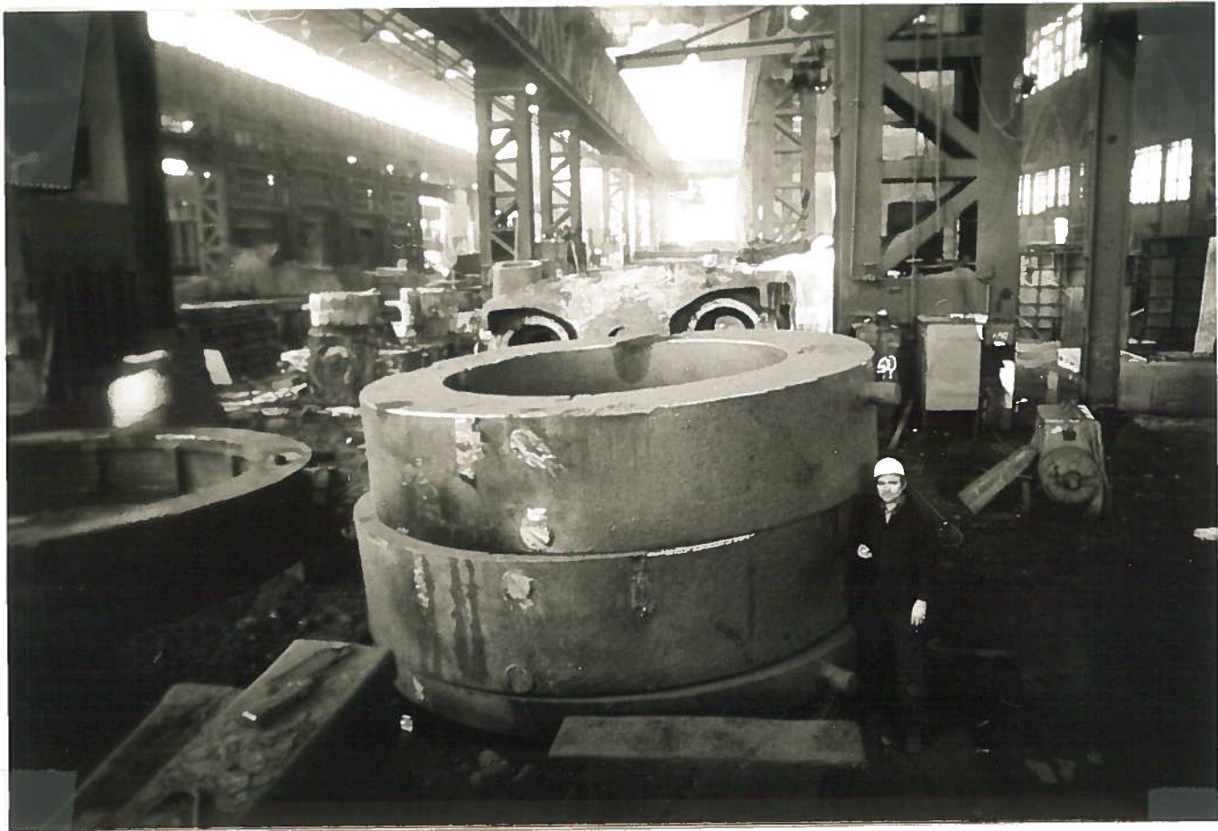
FIG. 20 - View of the rings after casting.
