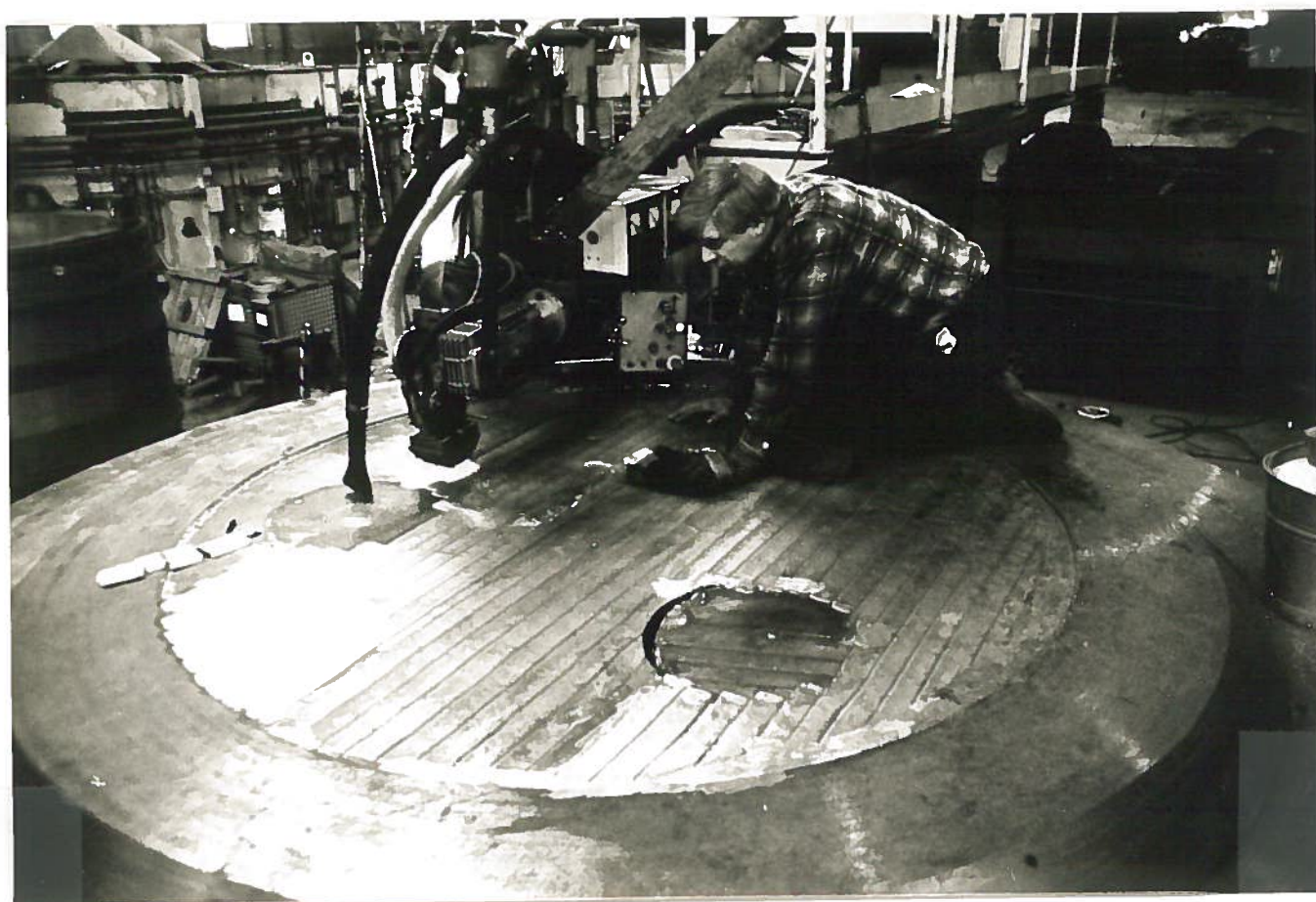
FIG. 25 - Welding of the stainless steel layer on the pole cap.
