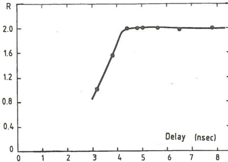
FIG. 9 - Double pulse resolution due to electronics only with a simulated input pulse.
