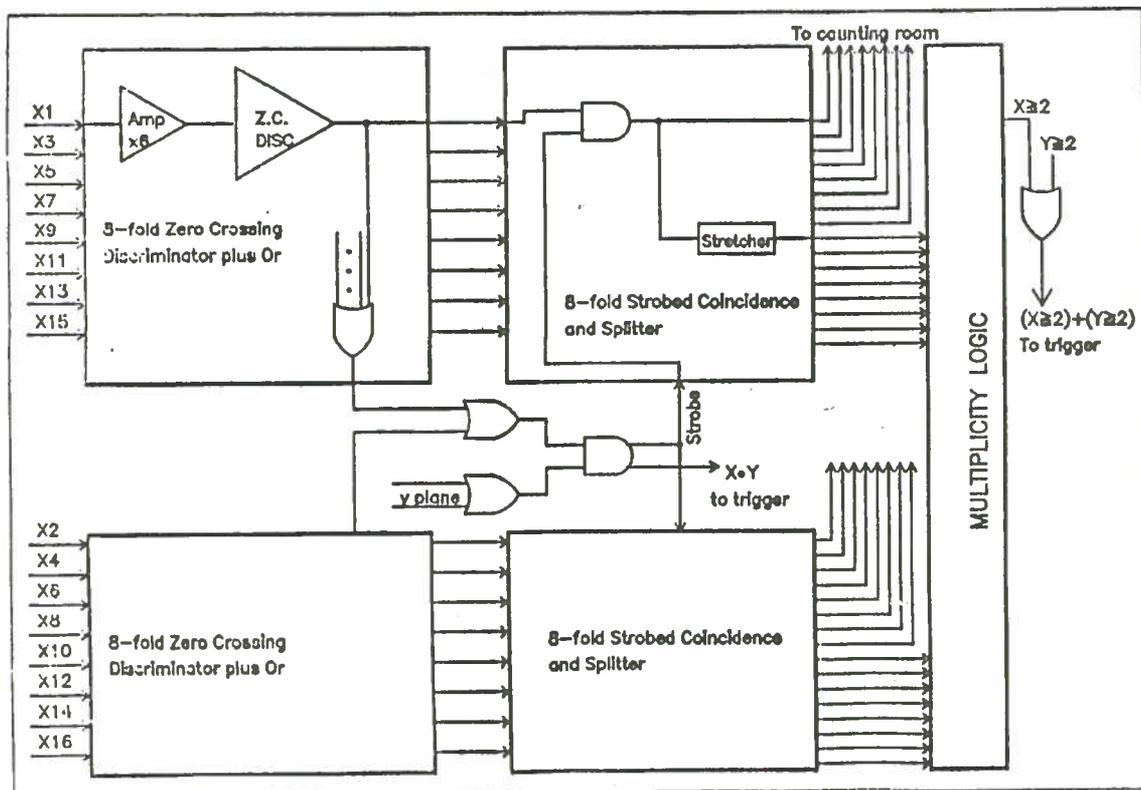
FIG. 2 - Block diagram of the close electronics.
