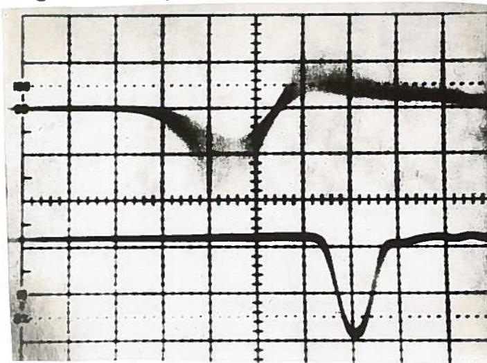
FIG. 3 - (top) Typical photomultiplier signals from a  $^{90}\text{Sr}$  source (20mV/div, 2 ns/div); (bottom) Zero crossing discriminator output signals (500mV/div, 2 ns/div. The oscilloscope is triggered on the zero crossing output signal).
