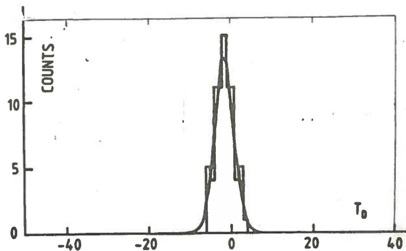
same time resolution for the two counters, a time resolution of 210 psec per counter is derived.
