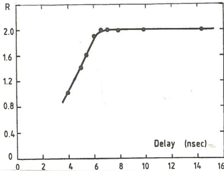
FIG. 8 - Double pulse resolution including the photomultiplier and the LED driving system.
