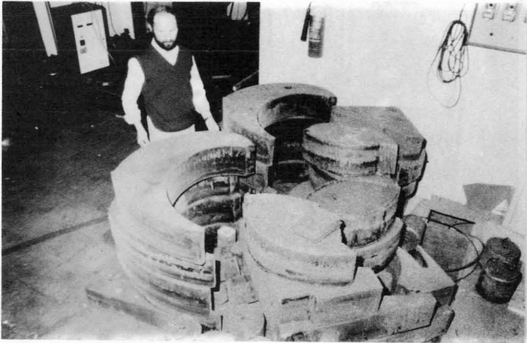
FIG. 13 - Flame-cut iron pieces for the sectors.
