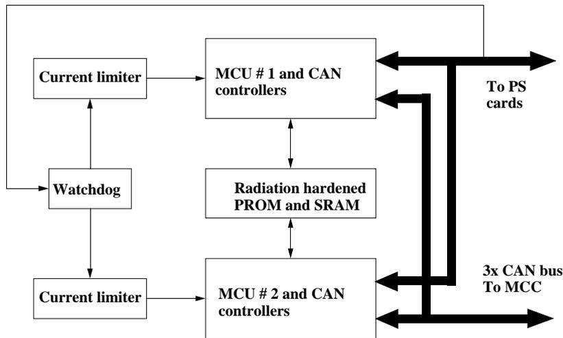
Figure 7: Block scheme of tracker power supply controller
