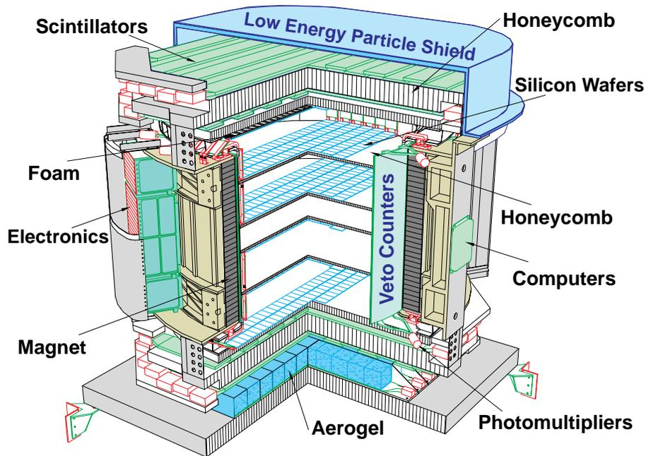
Figure 1: The AMS apparatus for the Shuttle flight STS-91
