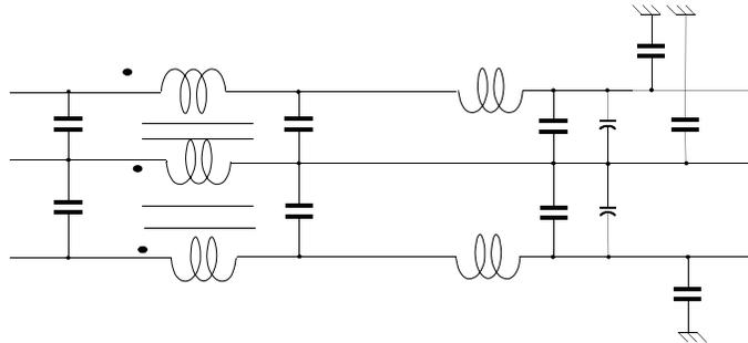
Figure 8: Most general filter configuration used at the output of each DC-DC converters, the value of each components changes in each configuration. In some configuration some components are missing
