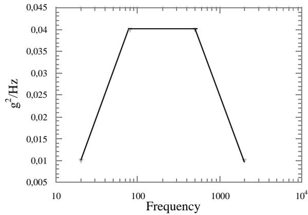
Figure 9: Random vibration test spectrum
