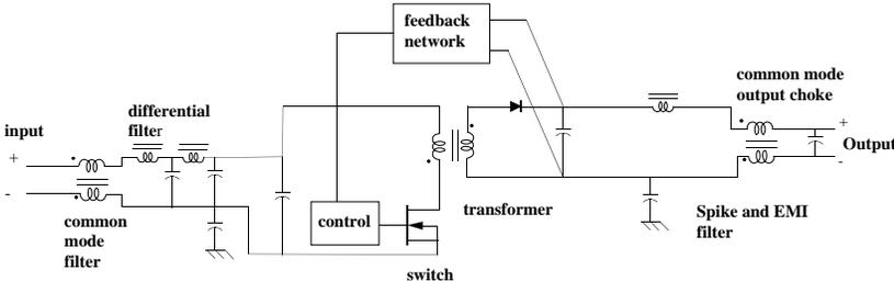
Figure 2: block scheme of an MDI DC-DC converter
