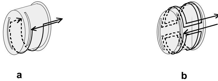
FIG. 4: The shape of the NMR coils for the NH 3 target and ND 3 target
