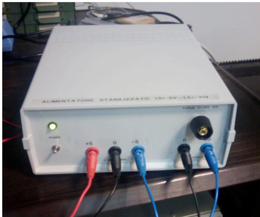
*Fig. 2: One of the dedicated, low-cost power supply to bias both the electronics and the APD sensor in each individual detection module.*
