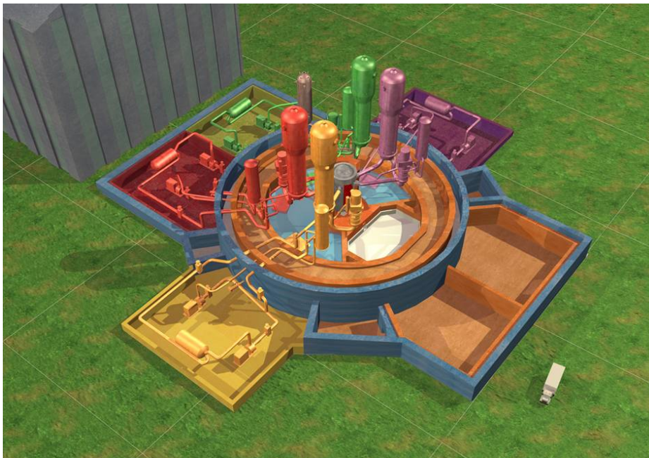
FIG 10a: Schematics of the nuclear island of EPR (European Pressurized water Reactor of AREVA-Siemens). This reactor of 1,6 GWe belongs to Gen III+ , and is inherently passive.
