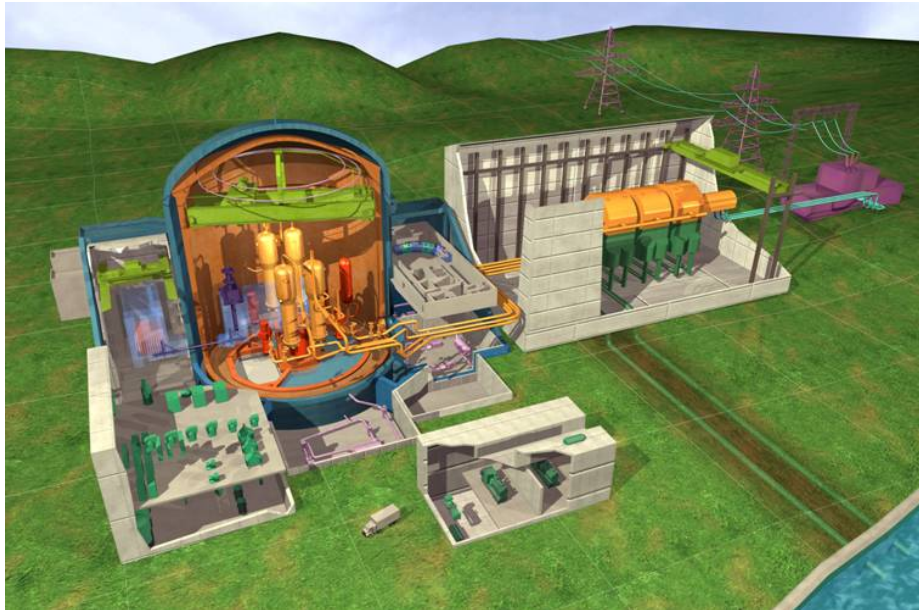
FIG 10b: Schematics of EPR , with turbine building and water cooling. No big cooling towers are necessary for the operation.
