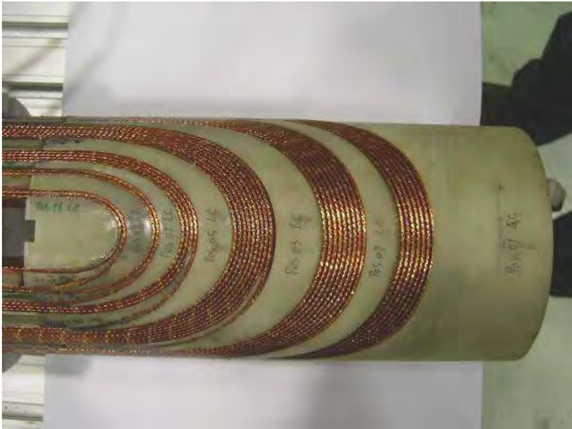
FIG.94: Details of the LC coil ends are shown. The 5 blocks result in 6 sections, being the larger one spitted into two parts.
