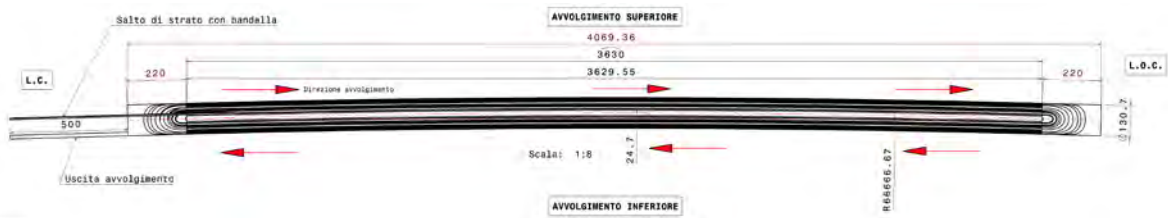
FIG.95: Longitudinal dimensions of the coil according to the design.
