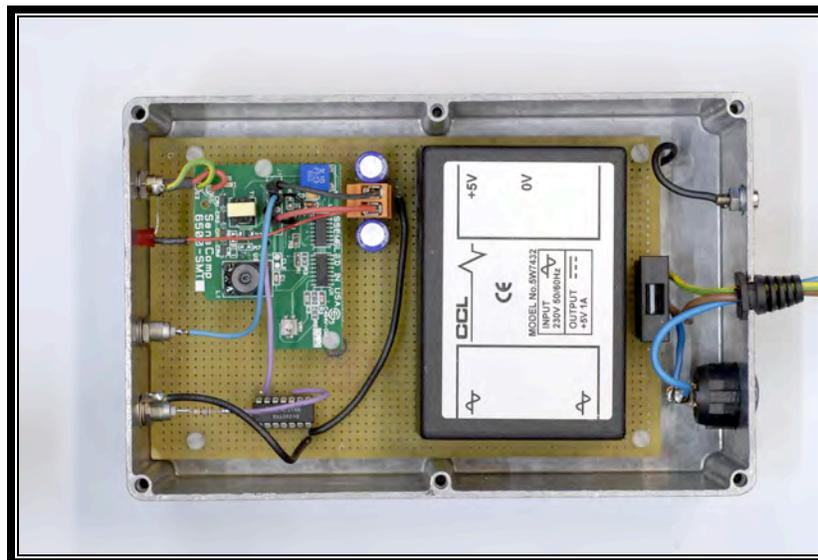
**Figure. 1.8** The Sonar Box with the electronics board
