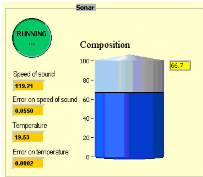
Figure 4.8: The Sonar System while running with 66.7 % of C4F10.
