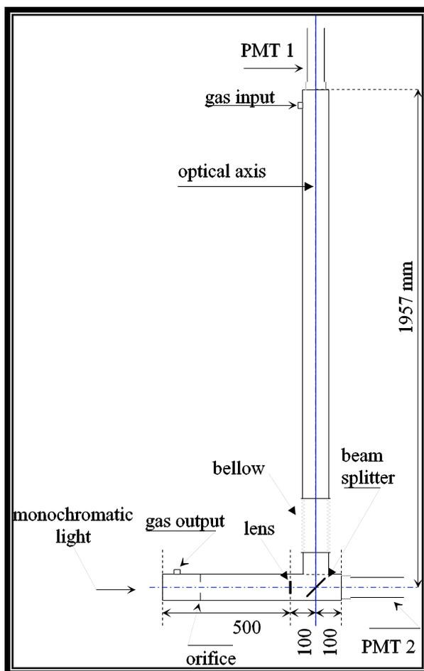
Figure 1.1 The monochromator gas tube
