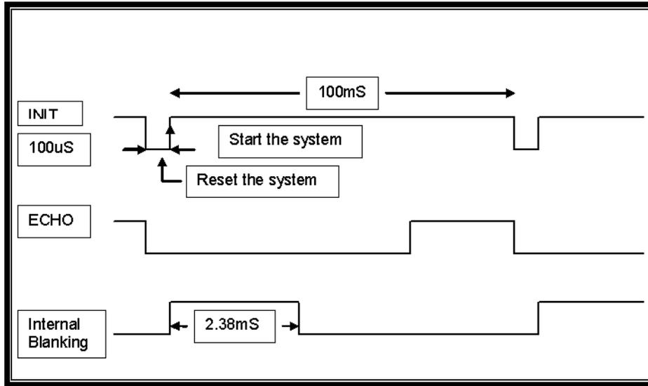
Figure. 1.9 Sonar signal timing
