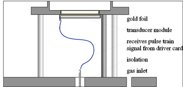
**Figure. 1.7** The Sonar System Setup
