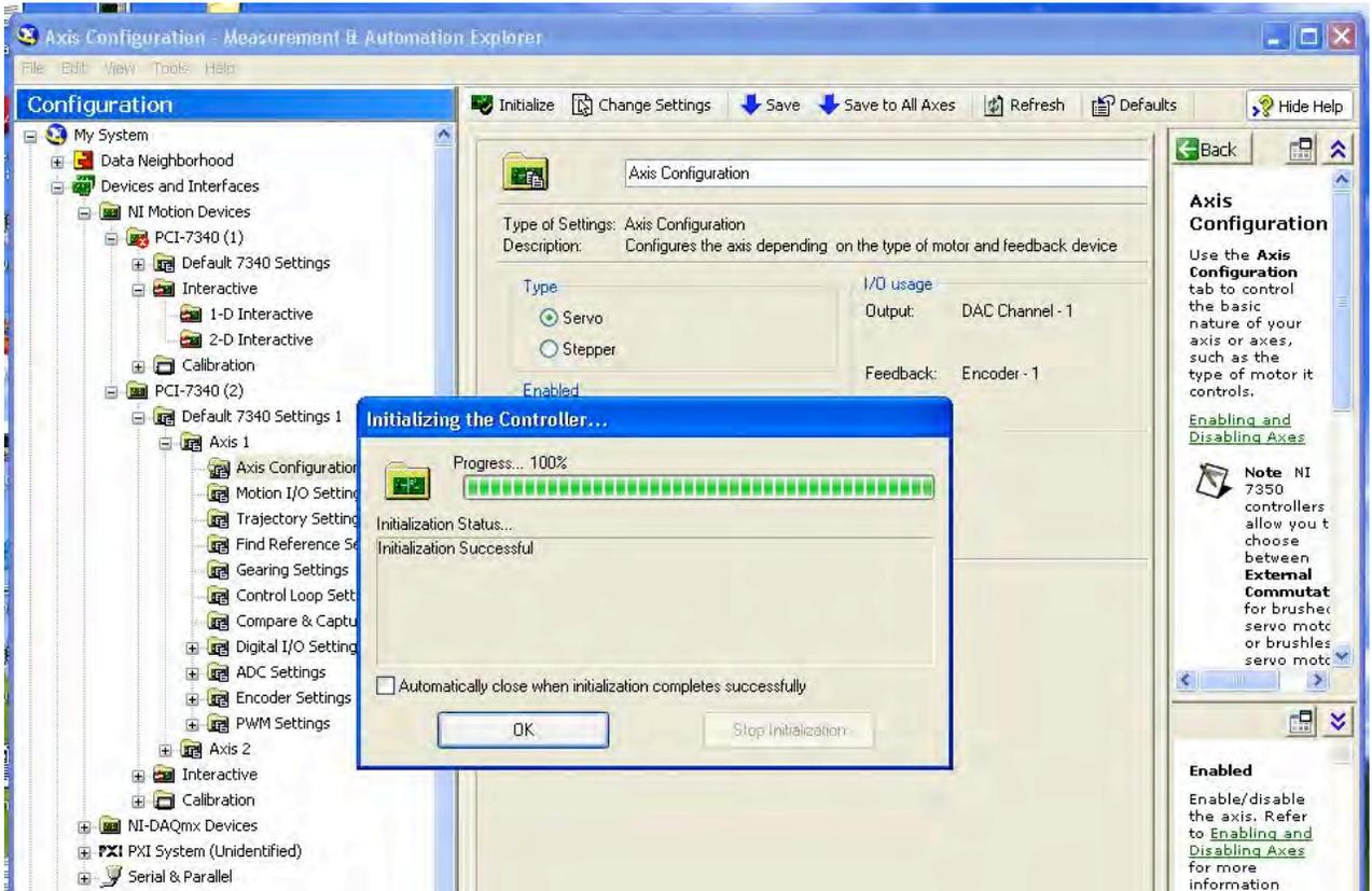
Figure 2.4: Initialization using MAX of NI MOTION controller
