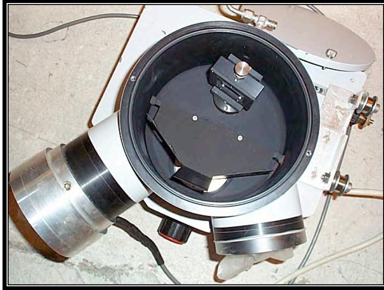
**Figure 1.2** McPherson model 234/302 monochromator
