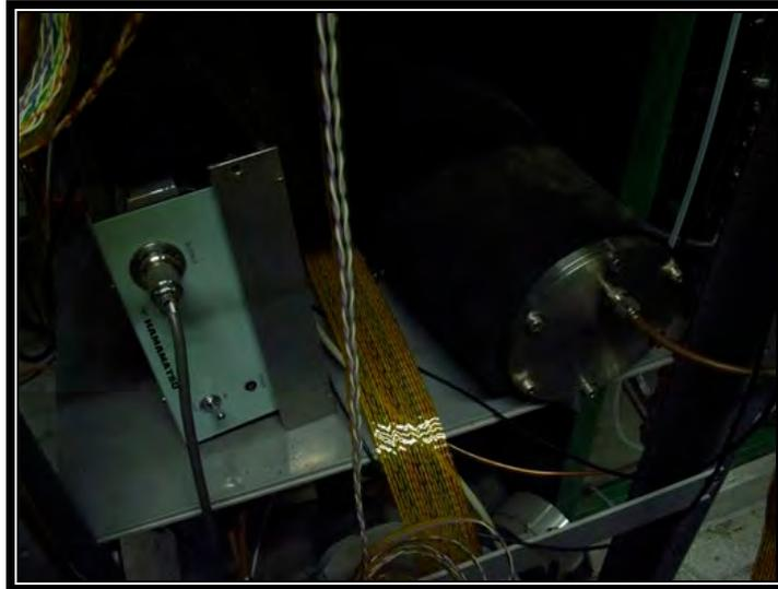
**Figure 3.5:** .- Monochromator Lamp power supply
