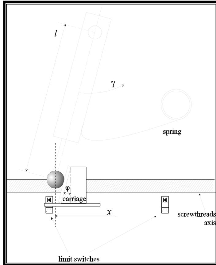
Figure. 1.3 The mechanical arrangement to steer the monochromator.
