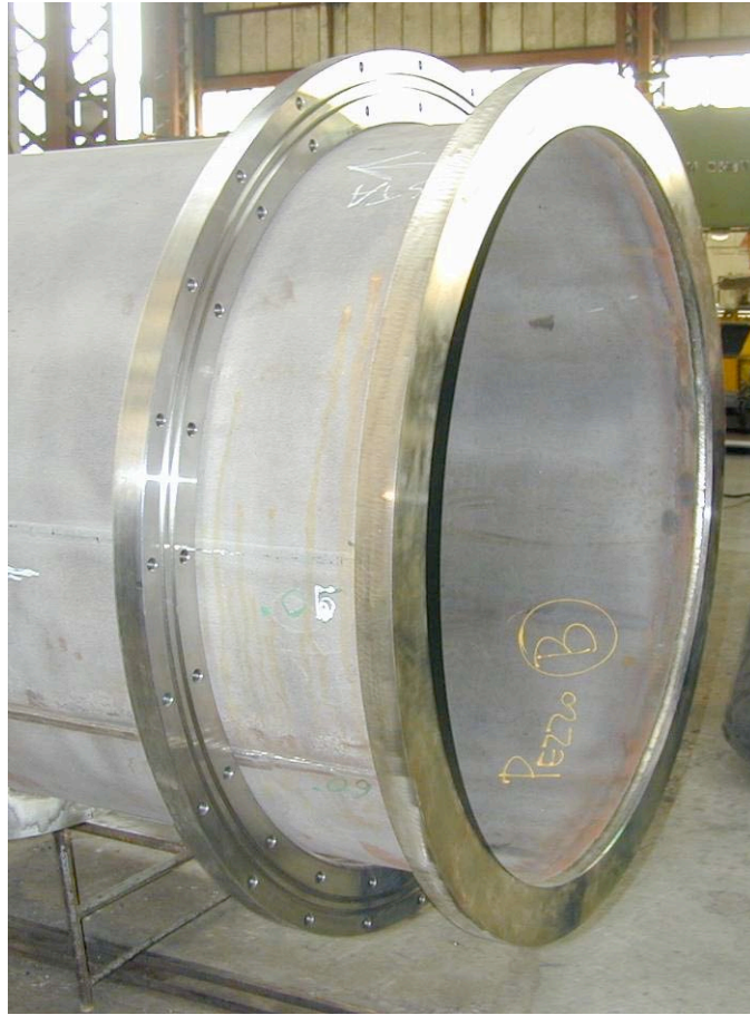
Figure 31: vacuum vessel in-flange
