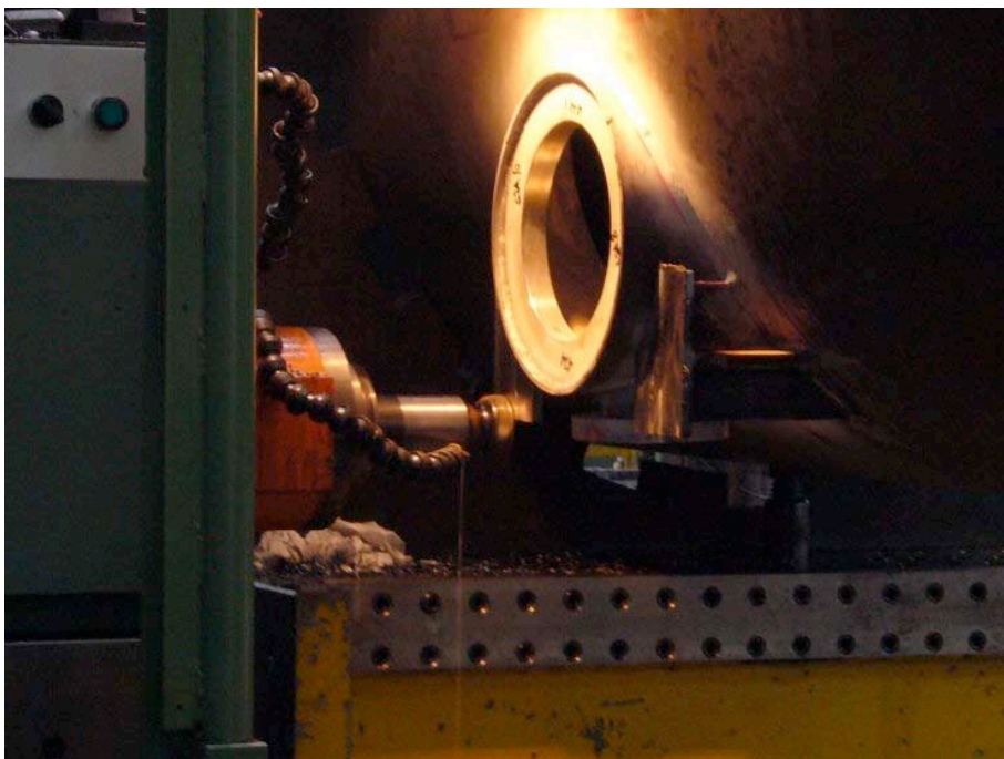
Figure 35: coupler flange machining
