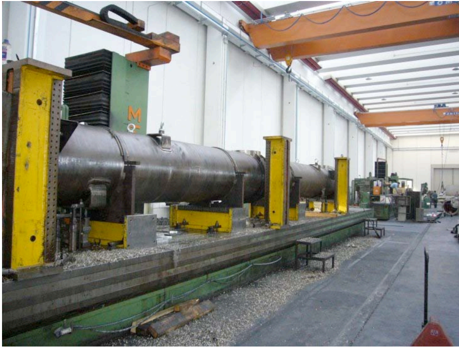
Figure 34: vacuum vessel positioning for final machining
