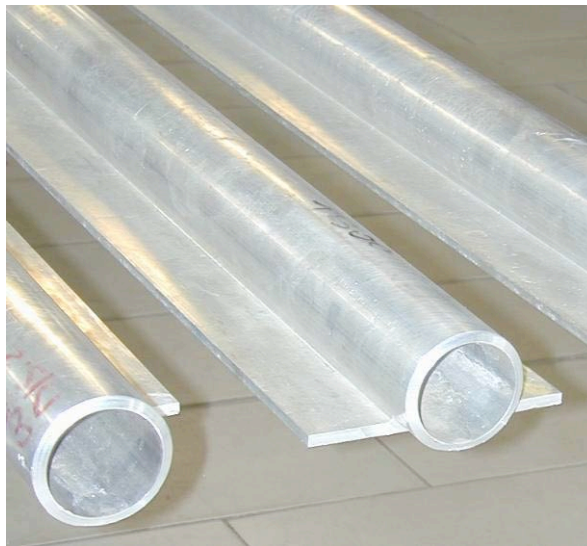
Figure 25: Al 5 K and 70 K return pipes
