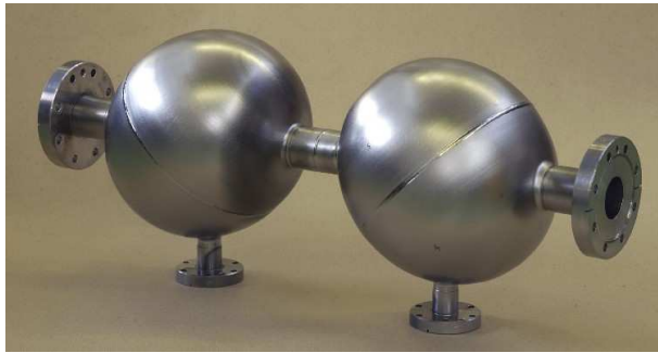
FIG. 2: Niobium spherical cavities (fixed coupling)
