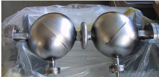
FIG. 3: Niobium spherical cavities (variable coupling)
