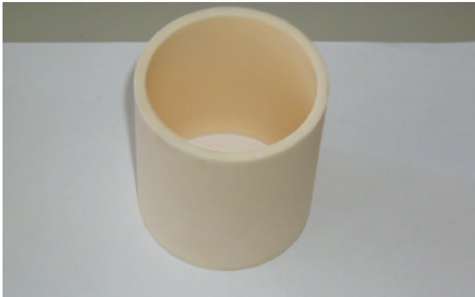
Figure 16. Allumina tube to be inserted in the TRIPS plasma chamber.
