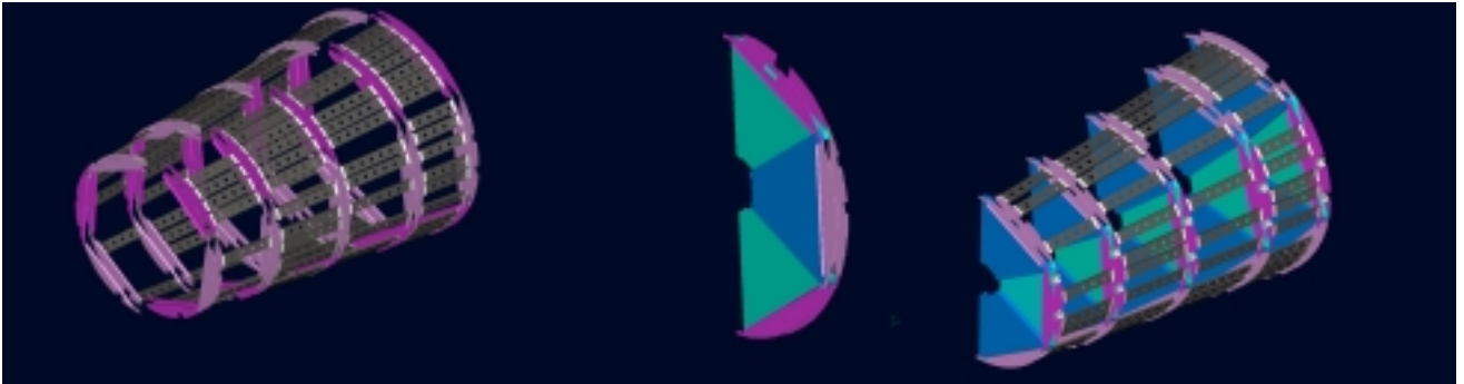
Fig. 10: skeleton frame concept: skeleton alone (left), a CSC plane inside the housing annulus (center), half T1 (right)
