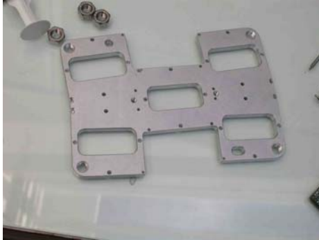
FIG. 12/a: "I" shaped module base-plate prototype, as manufactured FIG. 12/b: "I" shaped module base-plate prototype, with micro-cell base-board prototypes
