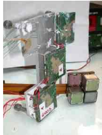
FIG. 12/a: "I" shaped module base-plate prototype, as manufactured FIG. 12/b: "I" shaped module base-plate prototype, with micro-cell base-board prototypes
