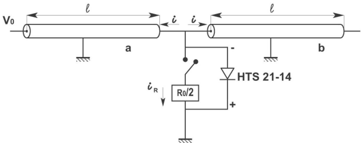
**Fig.4:** Schematic representation of the CPFL by different linear lines. HTS 21-14: transistor switch.
