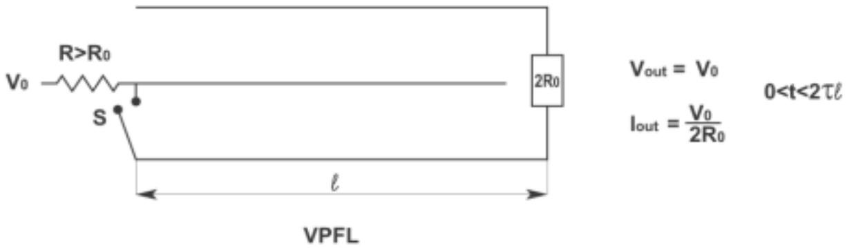
**Fig.2:** Schematic sketch of a voltage pulse forming line closed on its load impedance  $2R_0$ .
