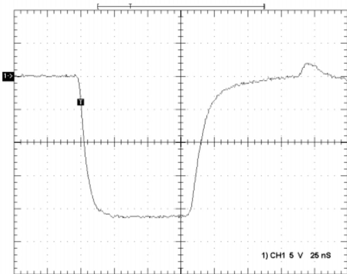
**Fig.5.** Waveform of the output voltage pulse recorded on the load  $R_{\phi}/2$ . Charging voltage 1kV output current 20A.
