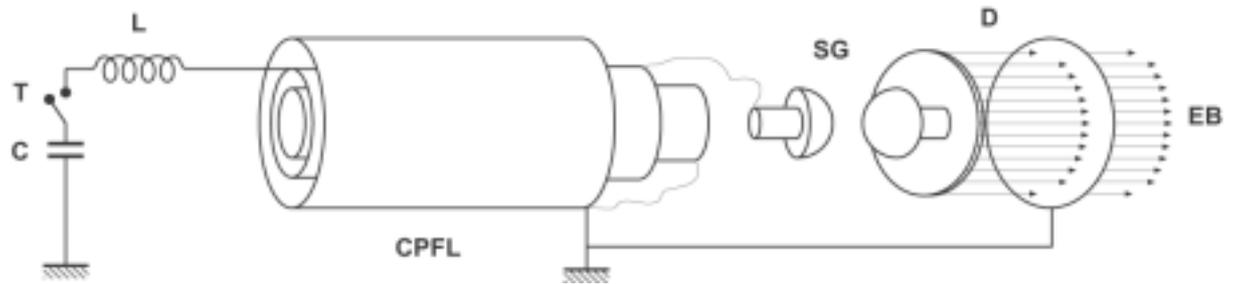
**Fig.7:** Schematic representation of a pulser halving the pulse width.
