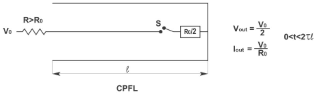
**Fig.3:** Schematic sketch of a current pulse forming line closed on its load impedance  $R_0/2$ .
