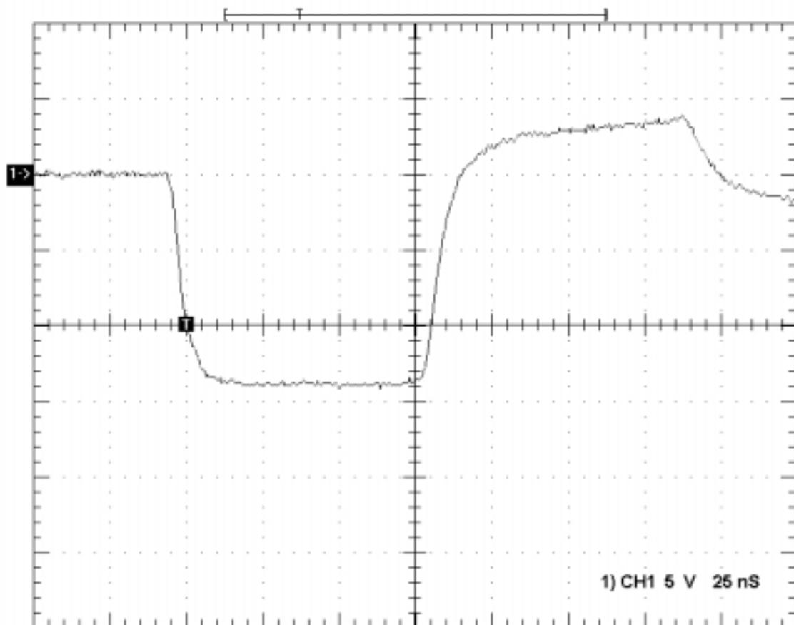
**Fig.6.** Waveform of the output voltage pulse recorded on the load  $R_{\phi}/2$  by one line. Charging voltage 1kV, output current 13.5A.
