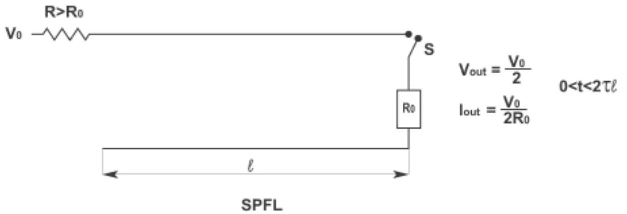
**Fig.1:** Schematic sketch of a single pulse forming line closed on its characteristic impedance  $R_0$ .
