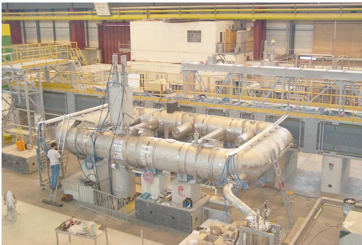
FIG. 1 – The B0 model coil in the test station at CERN.
