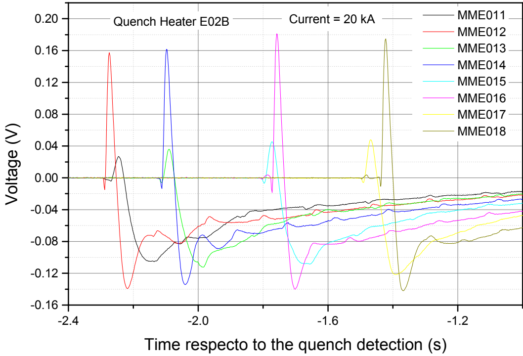
FIG. 18: Pick-up coil signals during a quench (main current = 20 kA).
