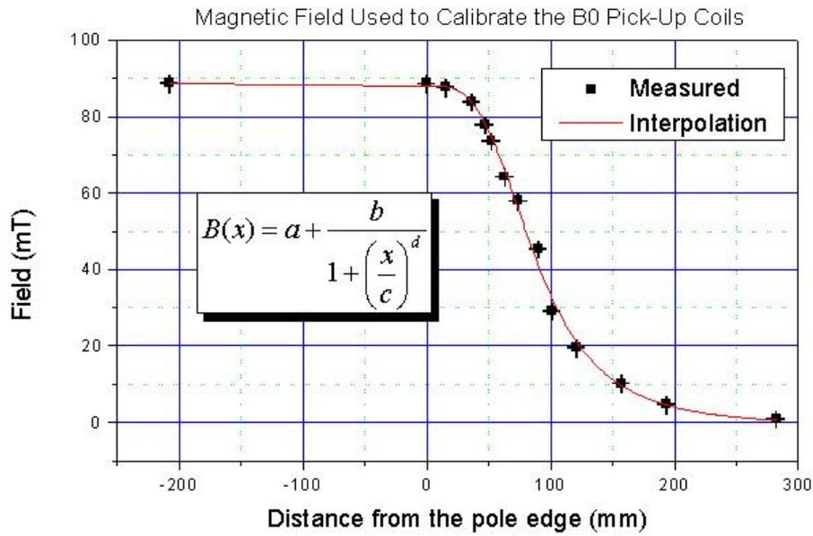
**FIG. 10:** The calibration magnetic field and the interpolation function
