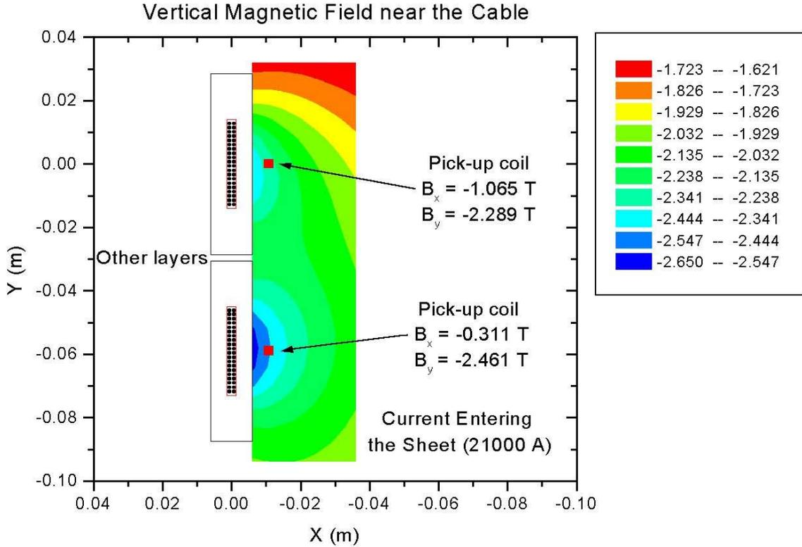
**FIG. 2:** Vertical component of the magnetic field around the B0 external cables.
