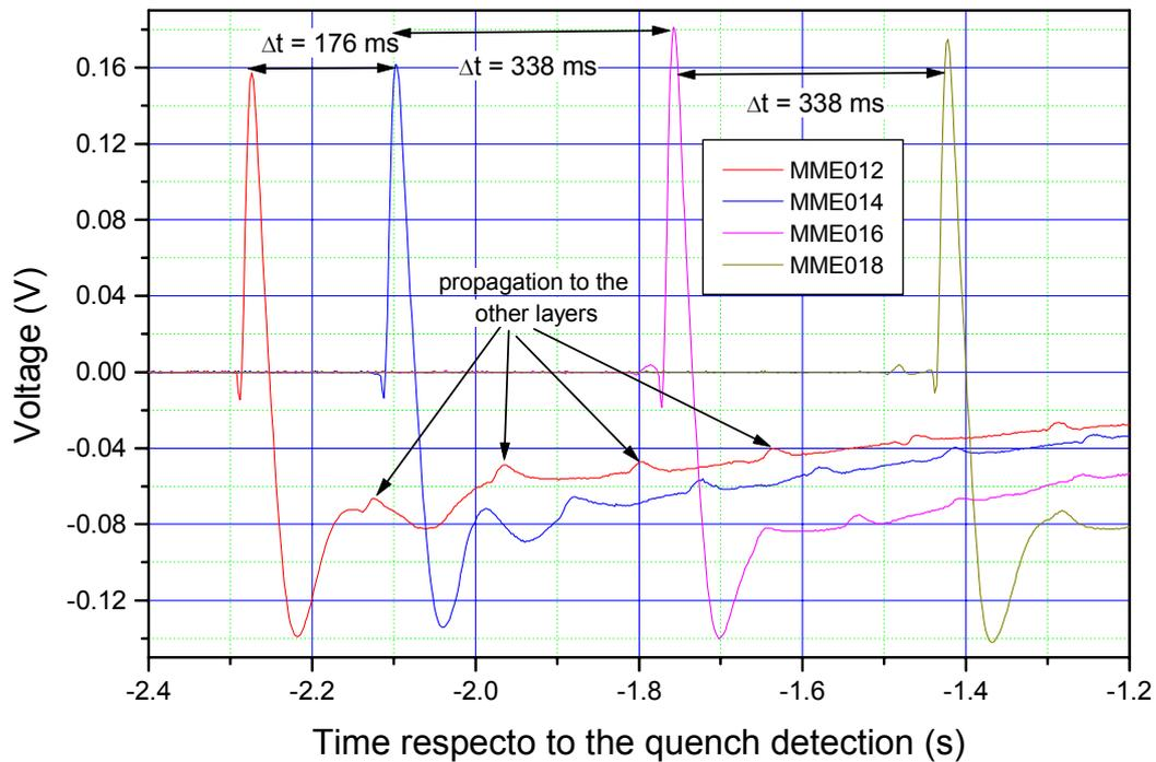
FIG. 15: Quench signal from the B0 pick-up coil
