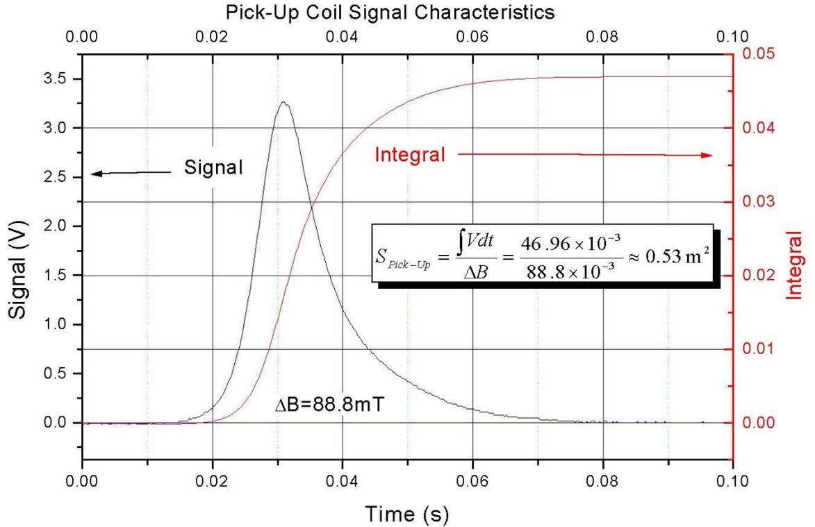
**FIG. 9:** Signal of the extraction from the calibration magnet with  $B = 88.8$  mT and the signal integral. The section indicated corresponds to this specific signal.
