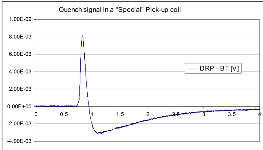
FIG. 14: Quench signal from a “special” pick-up coil
