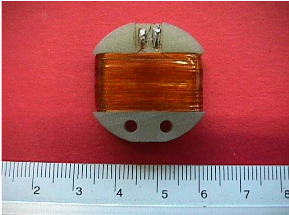
**FIG. 6:** A B0 pick-up coil
