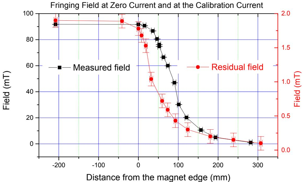
**FIG. 7:** The fringing field of the calibration magnet.
