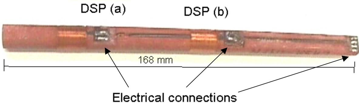
**FIG. 3:** The B00 DSP pick-up coil
