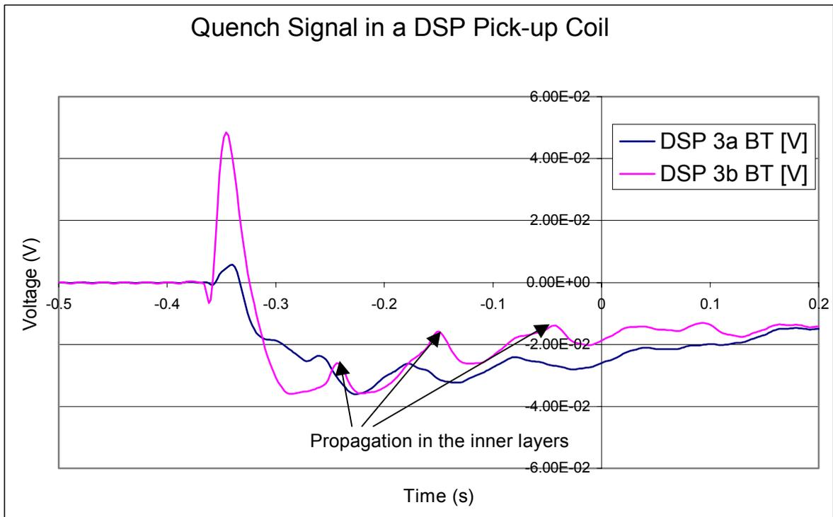
FIG. 12: Quench signal in the B00 DSP pick-up coil.
