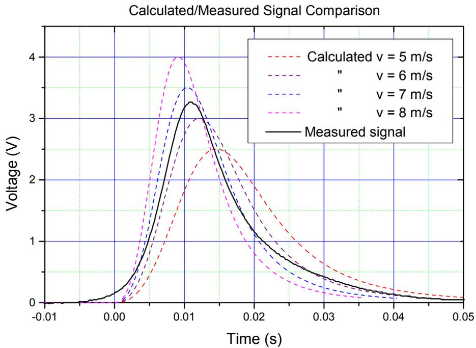
**FIG. 11:** Calculated pulse shape for different extraction velocities (dotted lines) and measured pulse (solid).
