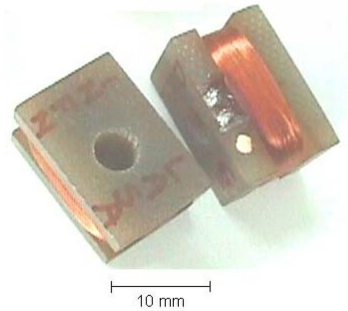
**FIG. 4:** The B00 DRP pick-up coil.
