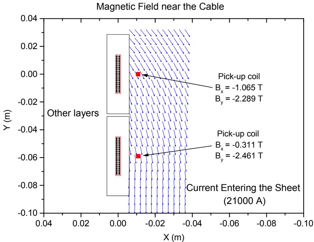
**FIG. 1:** Vector representation of the magnetic field around the B0 external cables.
