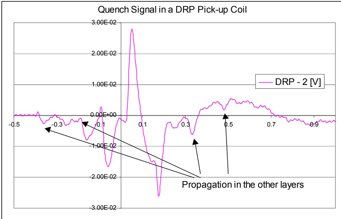
**FIG. 13:** Quench signal in the B00 DRP pick-up coil.
