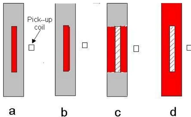
**FIG. 5:** Schematic representation of the current (red) diffusion from the superconductor to the stabilizer, during the quench.
