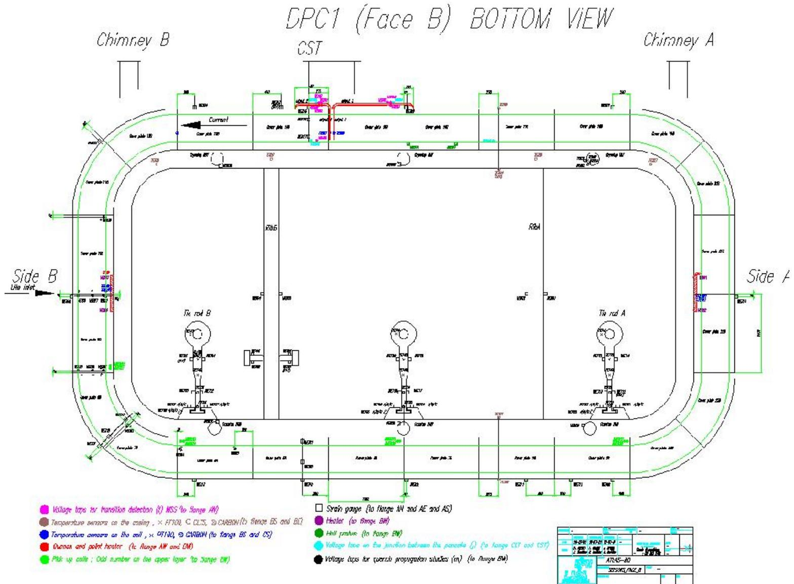
FIG. 1: Scheme of the sensor positions on the face B of the B0 coil casing.
