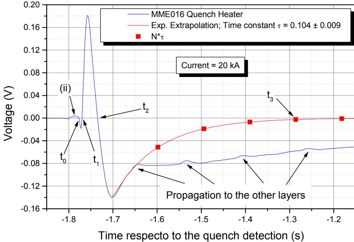
**FIG. 6:** Pick-up coil signal during a quench induced by a quench heater. The evolution of the diffusion process from the stabilizer to the current can be seen.
