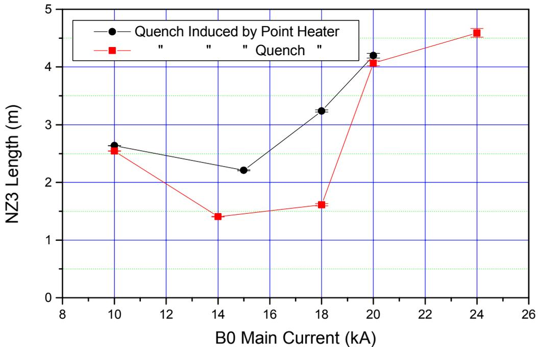
**FIG. 12:** NZ length of phase d) (vertical diffusion) at various main magnet currents for quenches induced by point heater (black) and quench heater (red).
