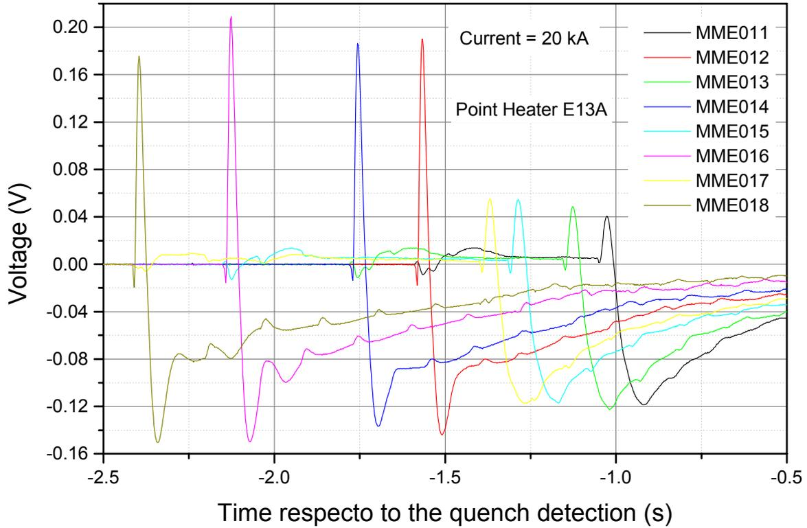
**FIG. 4:** Pick-up coil signals, quench induced by a point heater.
