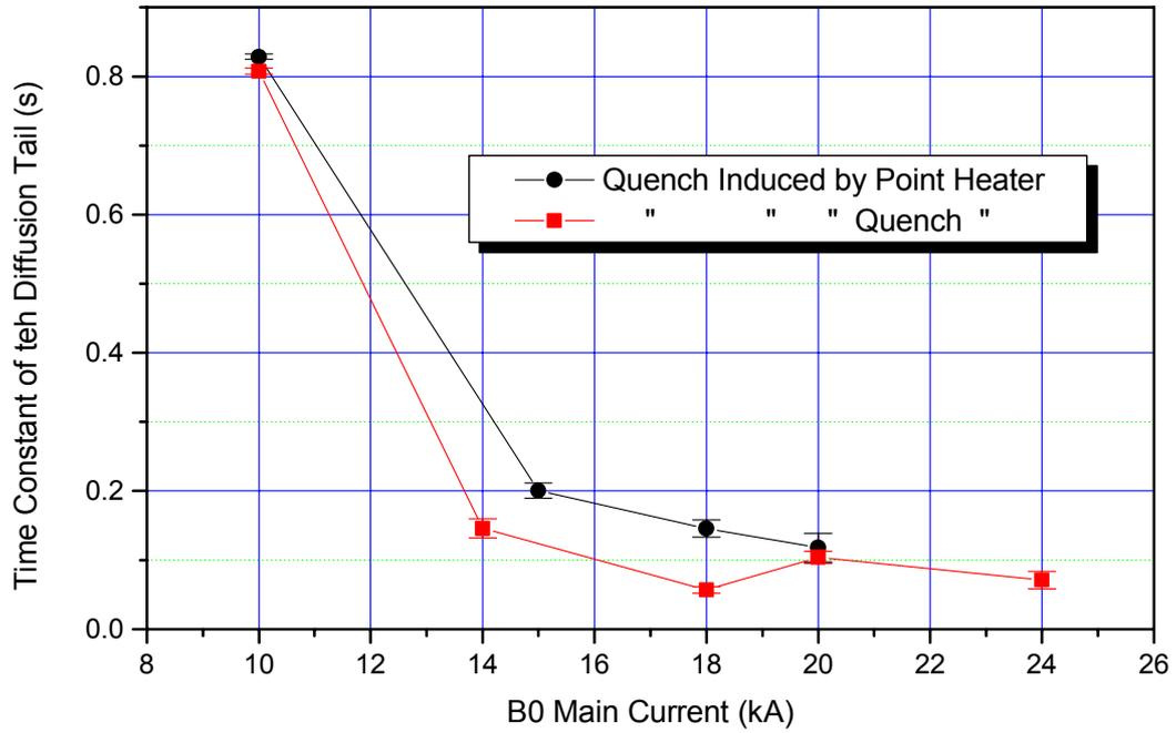
**FIG. 13:** Time constant of the exponential extrapolation of the tail of the pick-up coil signal (phase d) of the diffusion process).
