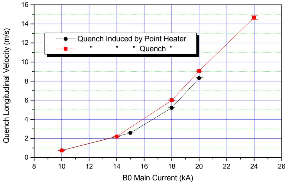
**FIG. 7:** Quench longitudinal propagation velocity at different current of the magnet, for quench induced by point heater (black) and quench heater (red).
