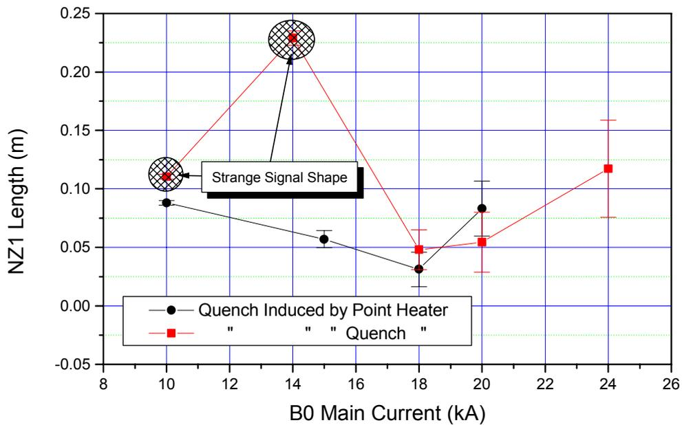
**FIG. 8:** NZ length of phase b) (partial horizontal diffusion) at various main magnet currents for quenches induced by point heater (black) and quench heater (red). (See text for details about the strange signals).
