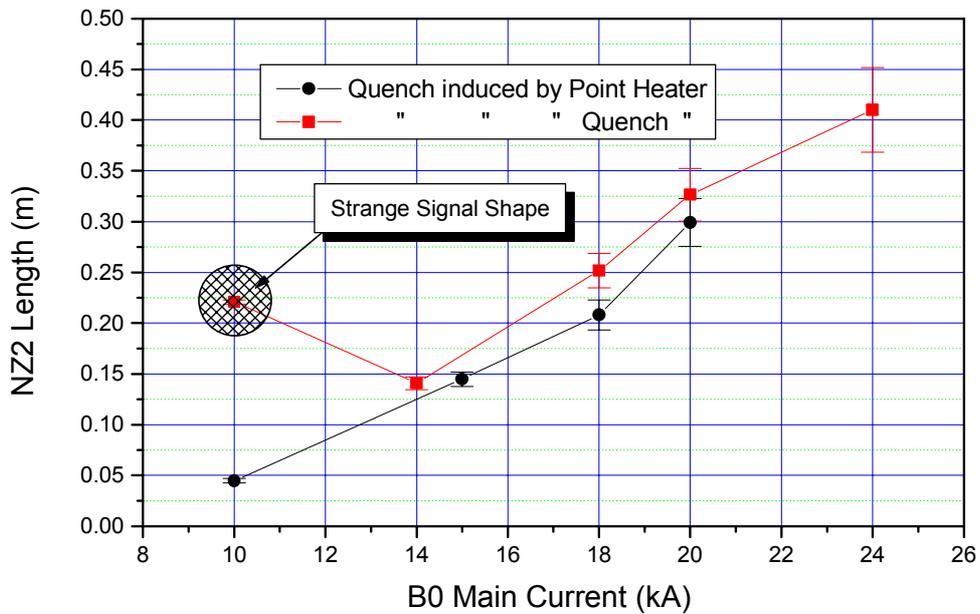
**FIG. 11:** NZ length of phase c) (horizontal diffusion) at various main magnet currents for quenches induced by point heater (black) and quench heater (red). (See text for details about the strange signals).
