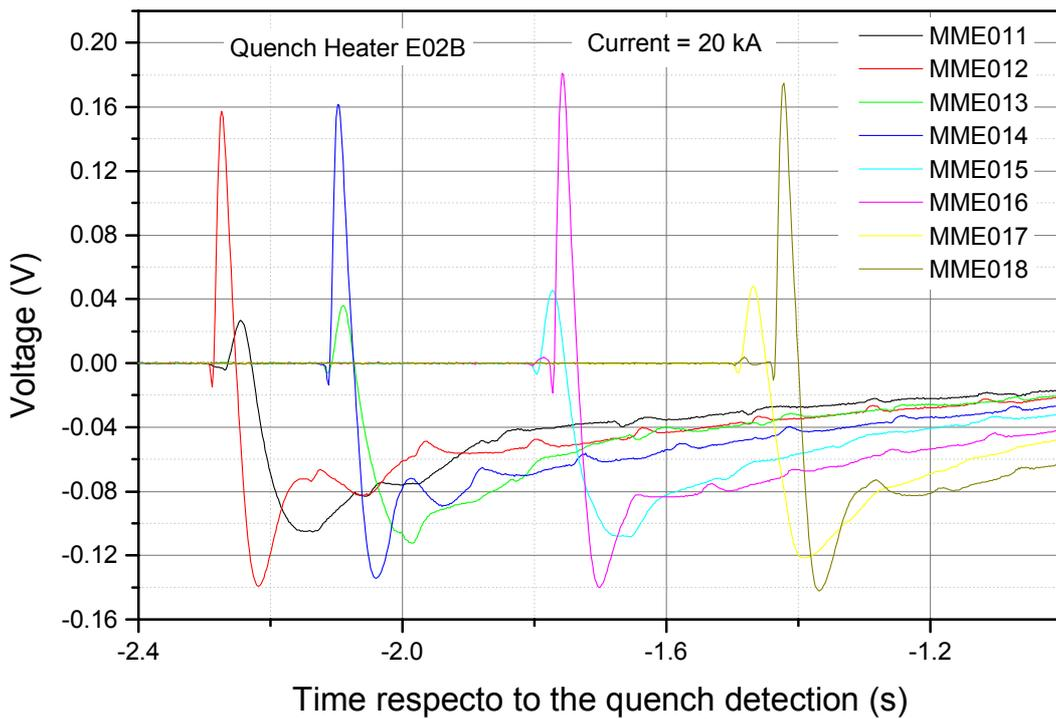
**FIG. 3:** Pick-up coil signals, quench induced by a quench heater.
