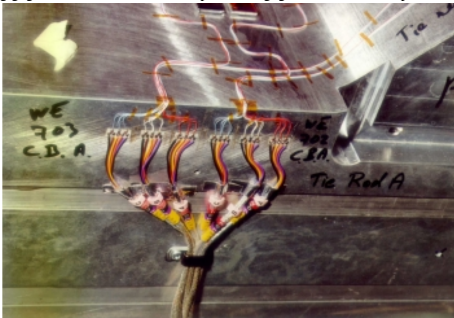
FIG. 7 – Strain gage WE703 of type SK-15-250-RA-350 mounted at the tie rod A root.
