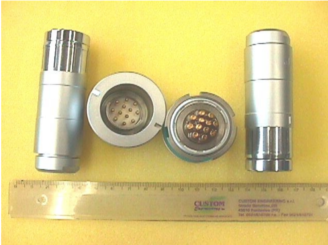
FIG. 12 – The 106 size connectors used in B0.
