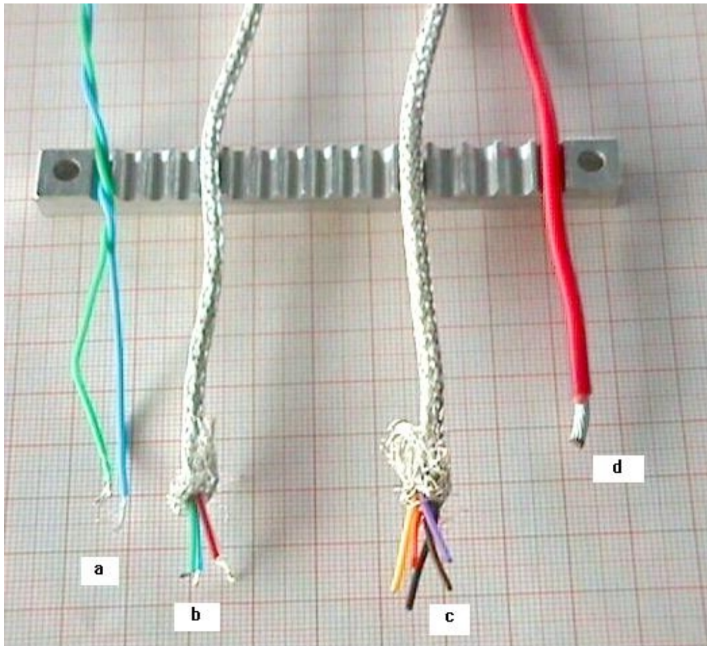
FIG. 11 – TInternal wiring cables.
