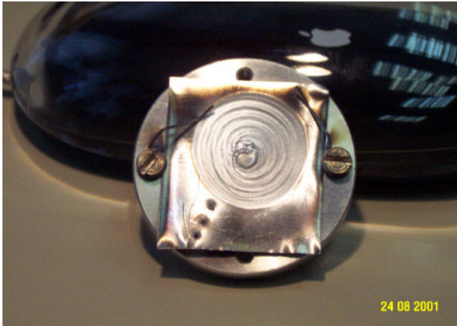
Fig. 35 - An Aluminum sample after 30 minutes of irradiation at 300 mJ, 30 Hz repetition rate.
