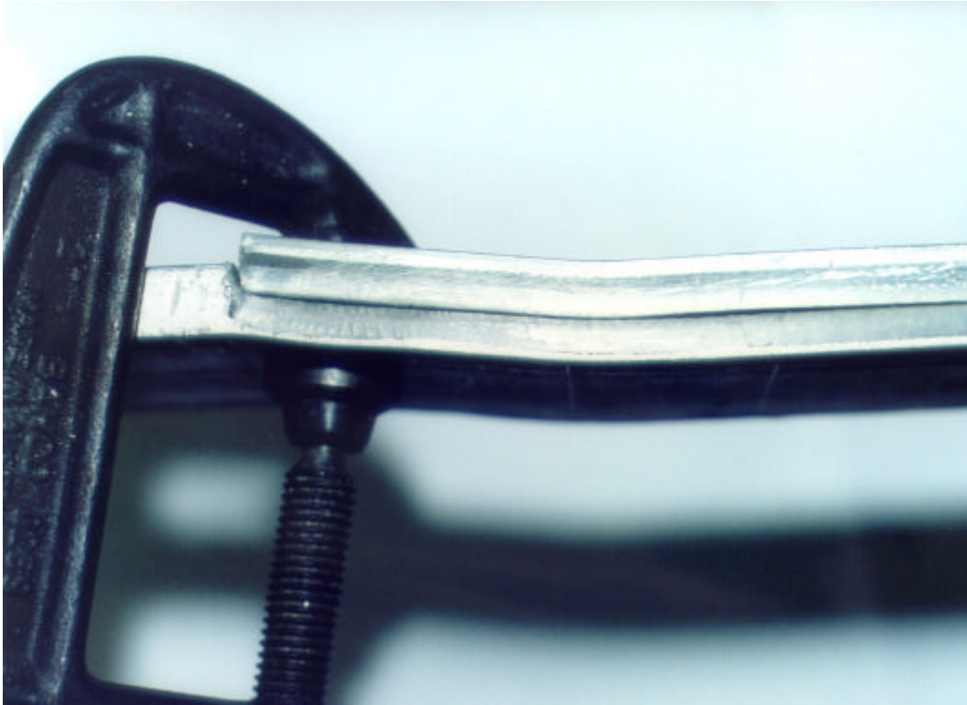
FIG. 3: The two pieces clamped in their final position, ready for welding.
