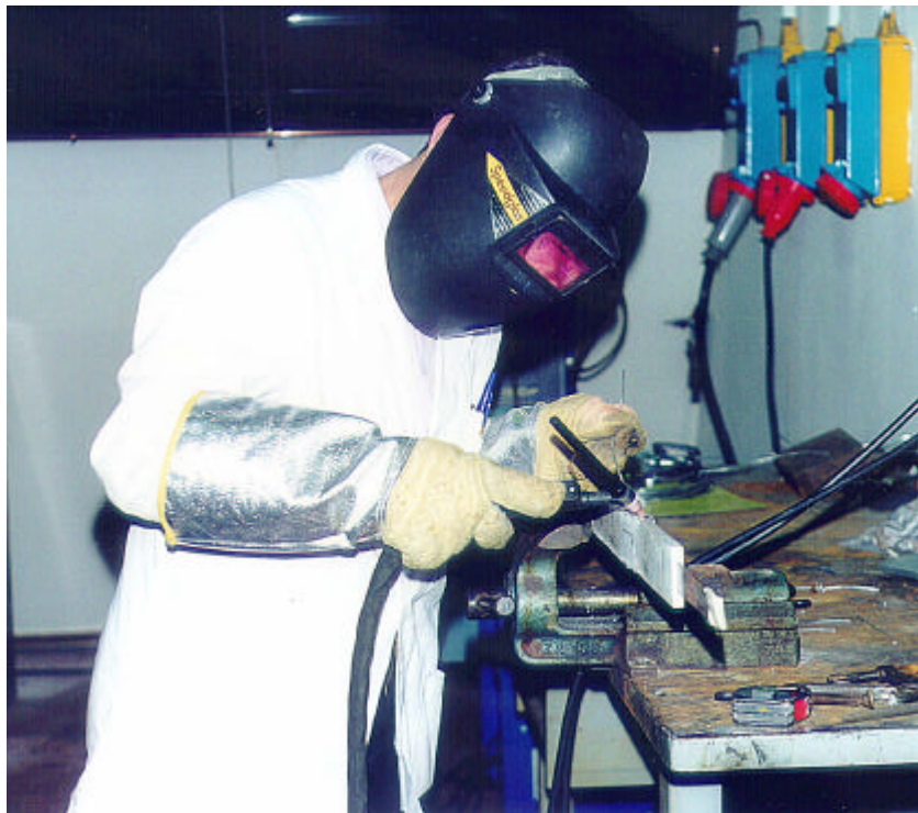
FIG. 4: TIG welding of the test joint.
