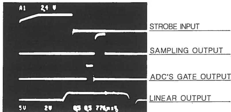
Fig. 7 - Photo of the timing of the 4 most significant pulses from the chain in fig. 6
