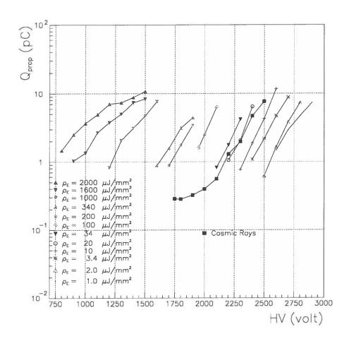
Figure 4: Pulse charge of the proportional tube as a function of HV for several laser intensities. The charge produced by cosmic rays is also shown (see text).
