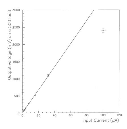
Figure 3: Calibration curve of the current amplifier used for the signal coming from the proportional tube. This device saturates the amplitude of the output signal at about  $2V/50\,\Omega$ .
