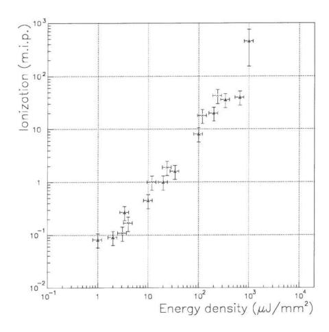
Figure 5: Ionization produced in the sensitive volume as a function of the energy density of the laser pulse. The stars and the triangles refers to two different data sets (see text).
