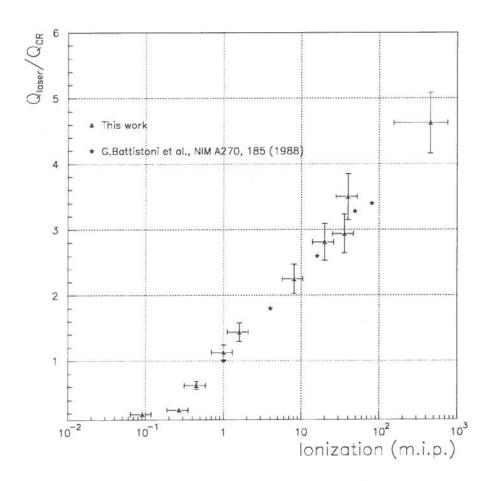
Figure 6: Streamer tube charge, HV=4200 V, divided by the charge produced by a cosmic ray, as a function of the primary ionization as measured by the proportional tube. Also shown, without the error bars, are the data obtained with high Z ion beams in [1].
