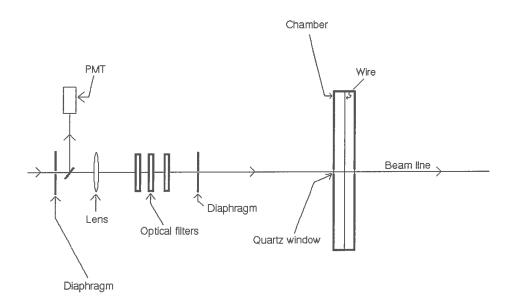
Figure 2: The experimental setup.
