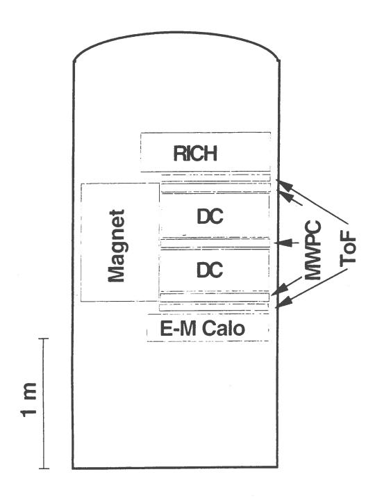
Fig. 1. Schematic diagram of the Wizard-CAPRICE apparatus used for the 1994 balloon flight to identify low energy cosmic ray antiprotons
