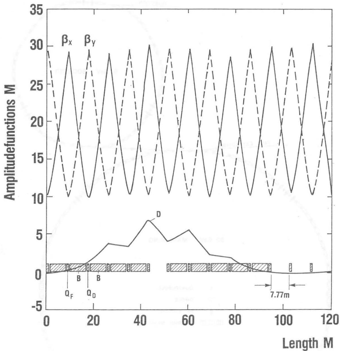
Fig. 6 - Proposed Lattice for the Main Ring. Also shown are the beta-functions in the horizontal and vertical planes and the dispersion function, for one superperiod.
