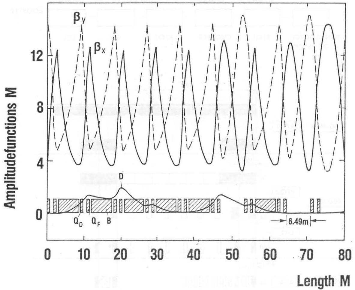
Fig. 5 - Proposed Lattice for the Booster Synchrotron. Also shown are the beta-functions in the horizontal and vertical planes and the dispersion function, for one superperiod.
