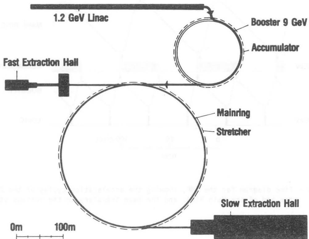
Fig. 1 - Schematic layout of the European Hadron Facility.
