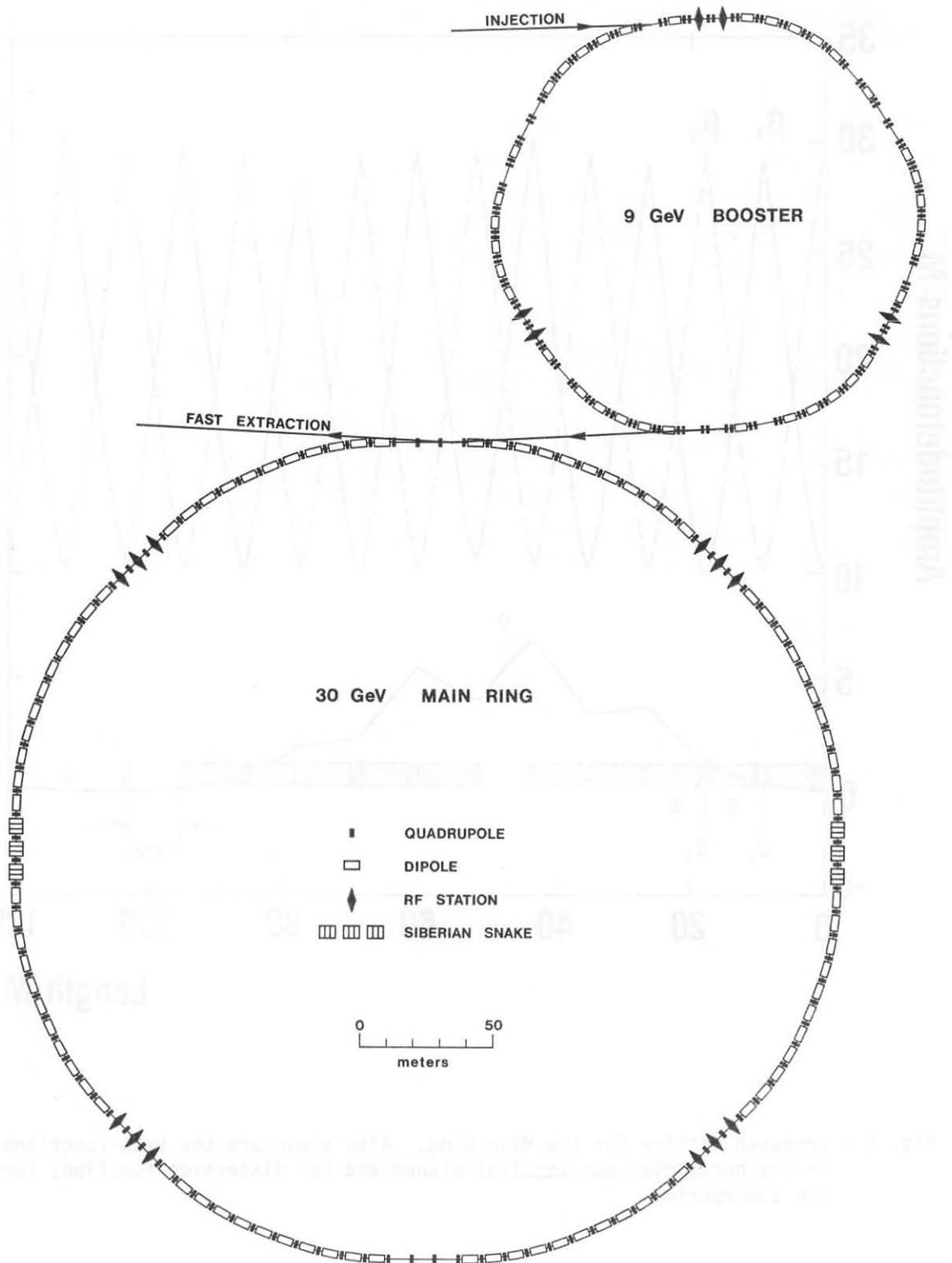
Fig. 7 - Arrangement of magnets and rf cavities for the Booster and Main Ring.
