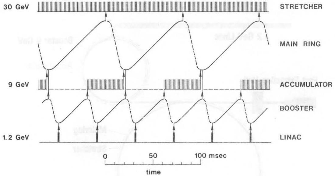
Fig. 2 - Time diagram for the EHF, showing the acceleration cycles of the Booster and of the Main Ring, and the beam transfers in the various stages.
