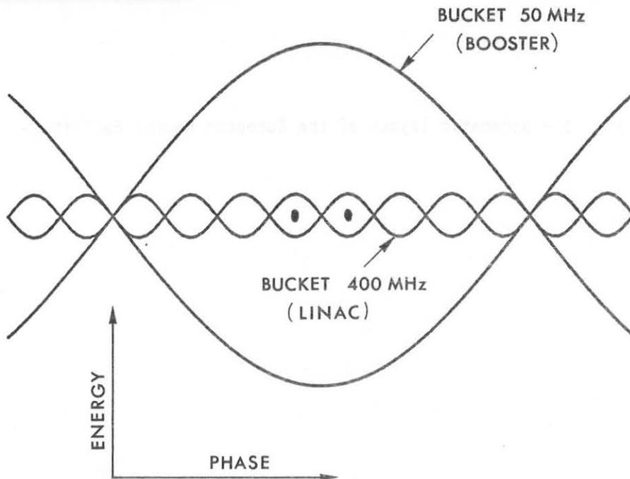
Fig. 3 - Longitudinal phase-space diagram showing the relative position of the LINAC bunches and the Booster bucket. By a suitable "painting" technique at injection 50% of the bucket area will be uniformly filled.
