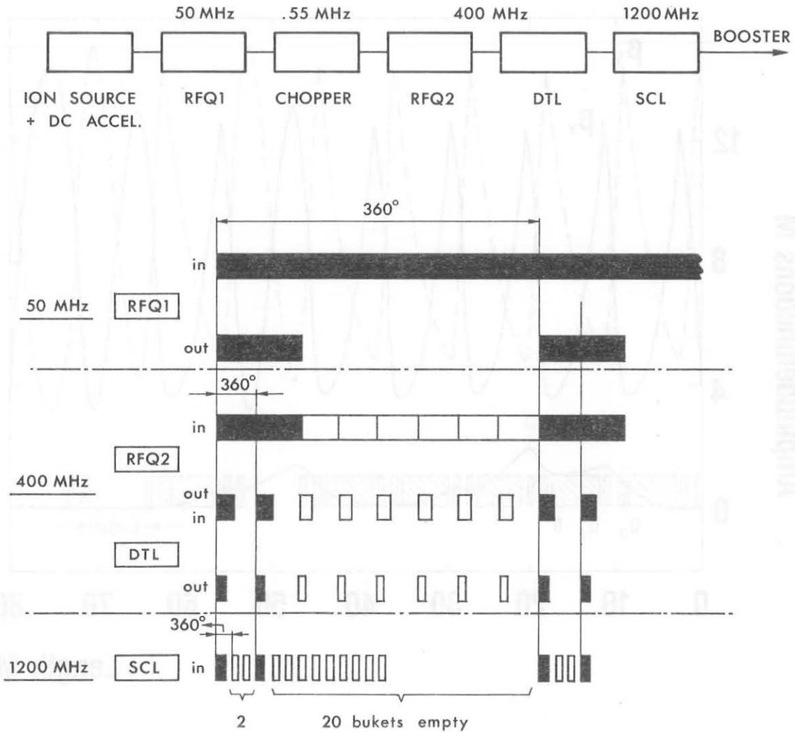
Fig. 4 - Schematic diagram of the Linear Accelerators and of the phase-compression of the d.c. beam from the ion source into the 2:8 bucket scheme for optimal injection into the Booster.
