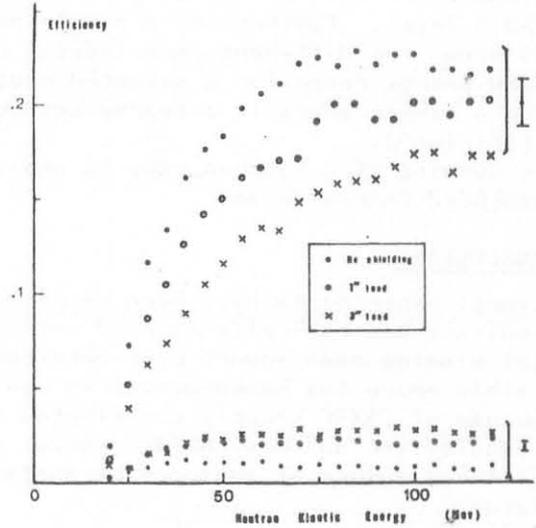
FIG. 8 - The upper experimental points show the overall detection efficiency of the module; the lower points show the absolute contribution of the "mixing".
