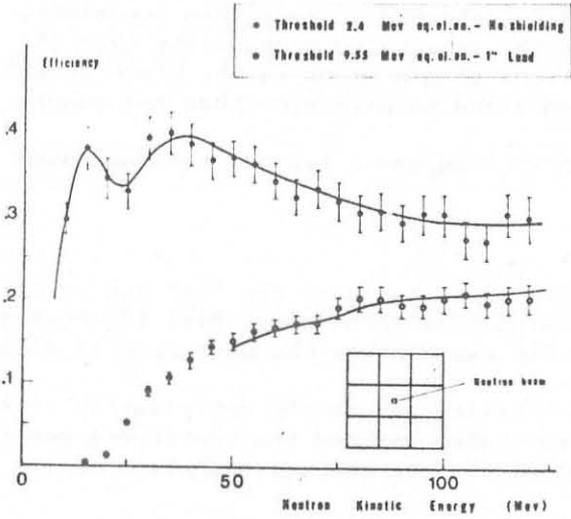
FIG. 7 - Efficiency of the 3x3 module for two different experimental conditions. In both cases the neutron beam was coincident with the central axis of the module.
