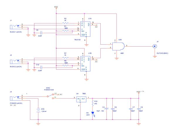
Fig.2: Lay-out of the coincidence circuit which may be used with two Geiger sensors to provide an output signal compatible with PASCO interfaces. Also shown is an optional power supply.
