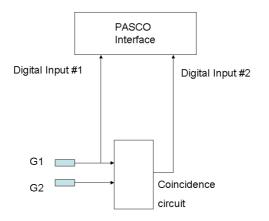
Fig.1: Sketch of the connections to the PASCO interface.
