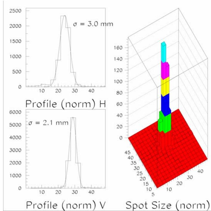
**FIG.3:** Vertical (Top) and horizontal (Bottom) profiles of the beam spot. The mean sizes ( $\sigma$ ), obtained from Gaussian fit are 3.0 mm and 2.1 mm respectively.
