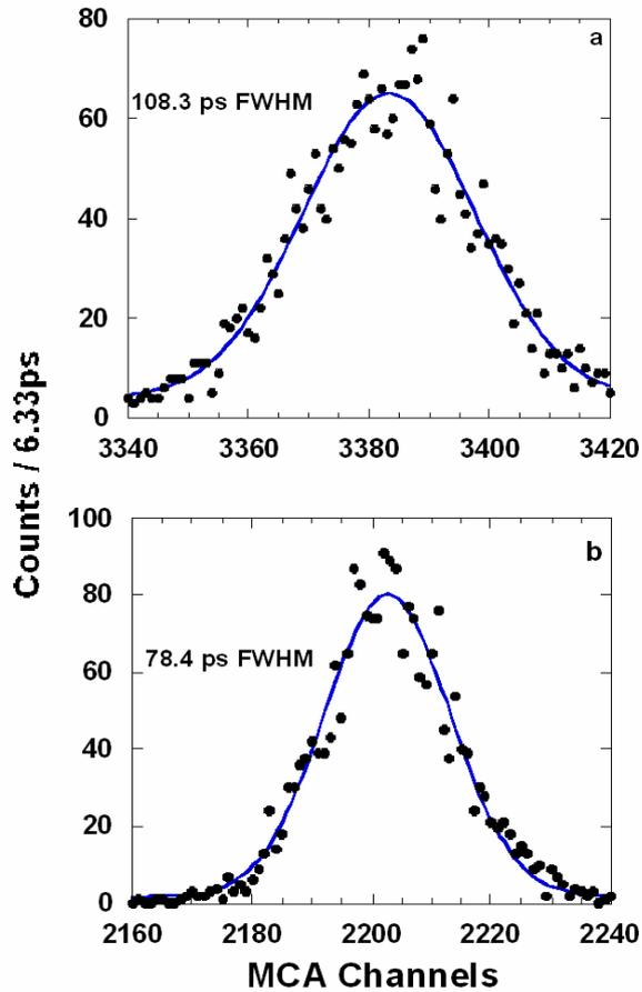
FIG. 5: Experimental data (Dots), and Gaussian best fit (Line) for BC408 (a) and BC404 (b).
