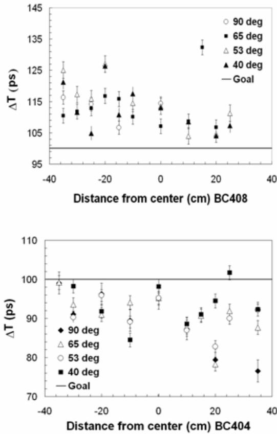
**FIG. 6:** The time resolution as a function of position (with respect to the center of the bar) at different impact angles, for BC408 (Top) and BC404 (Bottom). The solid line represents the expected limit resolution.
