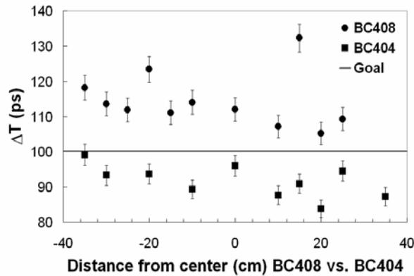
**FIG. 7:** Time resolution as a function of position, after averaging over the four impact angles for BC408 (dots) and BC404 (squares).
