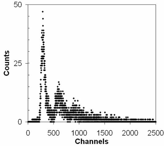
FIG. 4: Energy spectrum obtained by XP2020.
