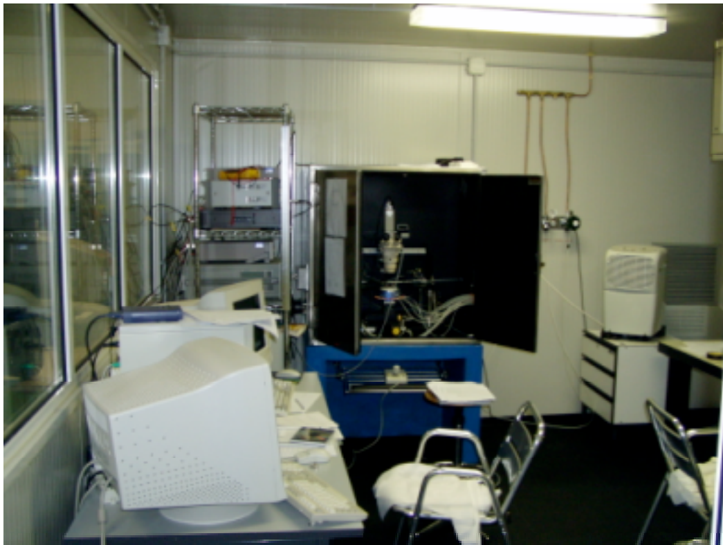
FIG. 3: The probe station and the dark box on the single block table.
