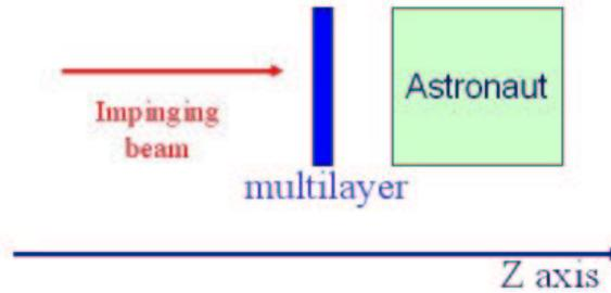
Figure 31: Experimental set-up: the primary particles impinge on the multilayer structure, the highest simplification of the SIH shown in fig. 30, and on the Astronaut.
