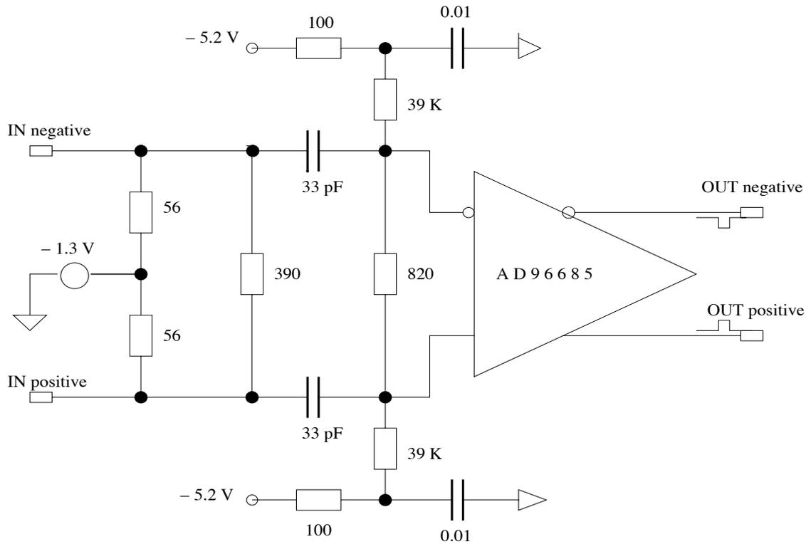
Figure 9: Line Receiver electronic circuit.
