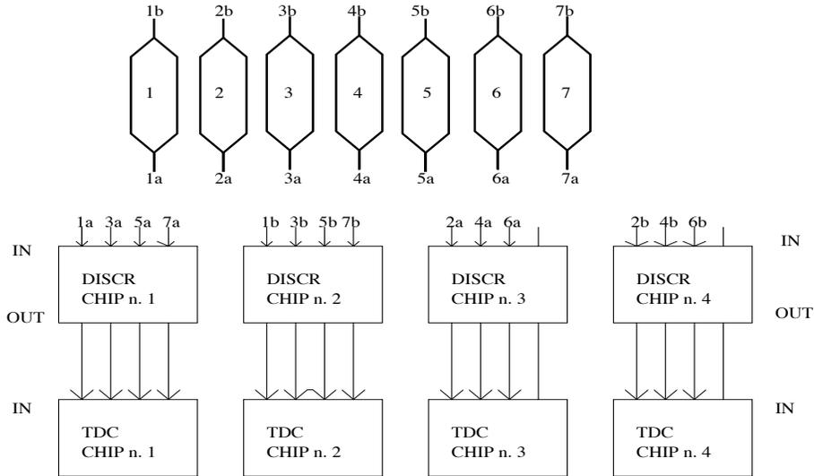
Figure 3: Cabling scheme. Each palisade is subdivided in 2 groups of 7 and 6 scintillator slabs (top panel). Signal from PM coming from the same slab are fed to discriminator channels located in different chips (bottom panel) to minimize the crosstalk. The 4 DISCR chips belong to the same discriminator LECROY 4413. The 4 TDC chips belong to the same TDC VME CAEN V775.
