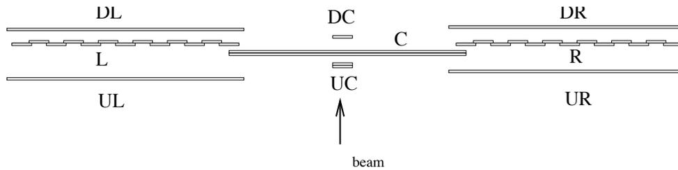
Figure 14: A cross section of the TOF-WALL showing also the adopted naming scheme. Also the ancillary upstream counters are shown.
