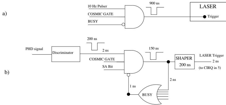
Figure 18: The generation of the laser pulse a) and the logic to produce a laser trigger b).
