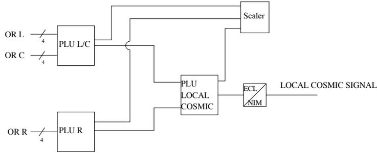
Figure 16: The cascade of the PLU generating the signal of a cosmic crossing the Up-stream Downstream counters and possibly also the TW.
