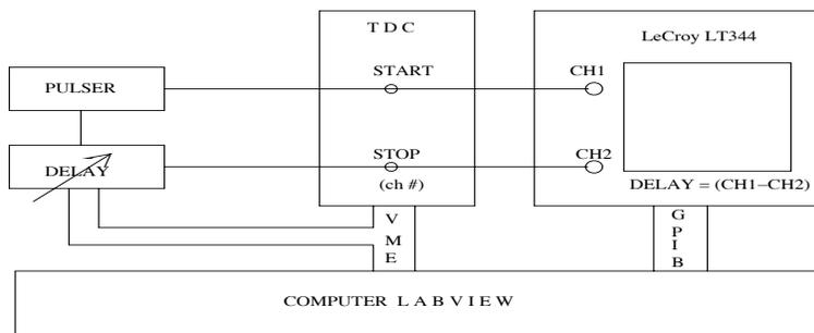
Figure 10: Setup scheme of TDC linearity measurement.
