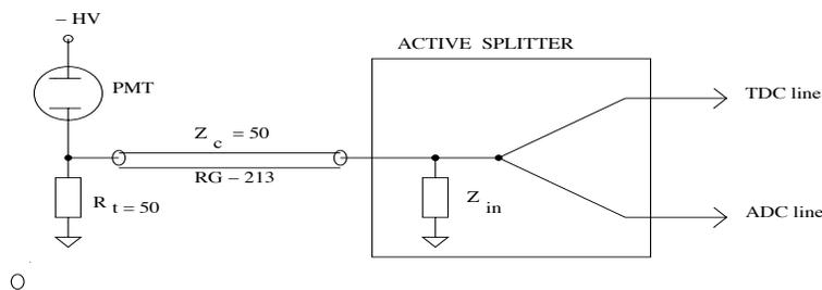
Figure 4: Active splitter impedance matching scheme.
