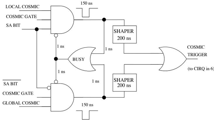
Figure 17: The logic implemented to generate the Cosmic Trigger and selection of local vs global cosmic signal.
