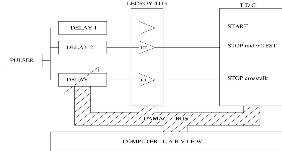
Figure 6: Setup scheme of crosstalk measurement.
