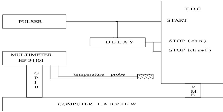
Figure 13: Setup scheme of TDC measurement allowing temperature variation.
