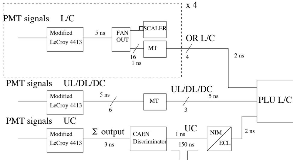
Figure 15: Sketch of the treatment of the PM signals in the Left and Central palisades to generate a local cosmic trigger.
