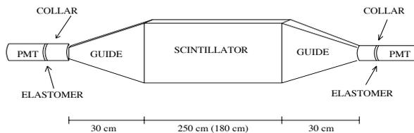
Figure 1: HARP TOF-WALL counter with readout at both ends.
