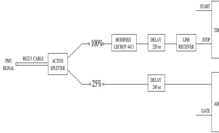
Figure 2: Block diagram showing the processing and conversion of PM signals.
