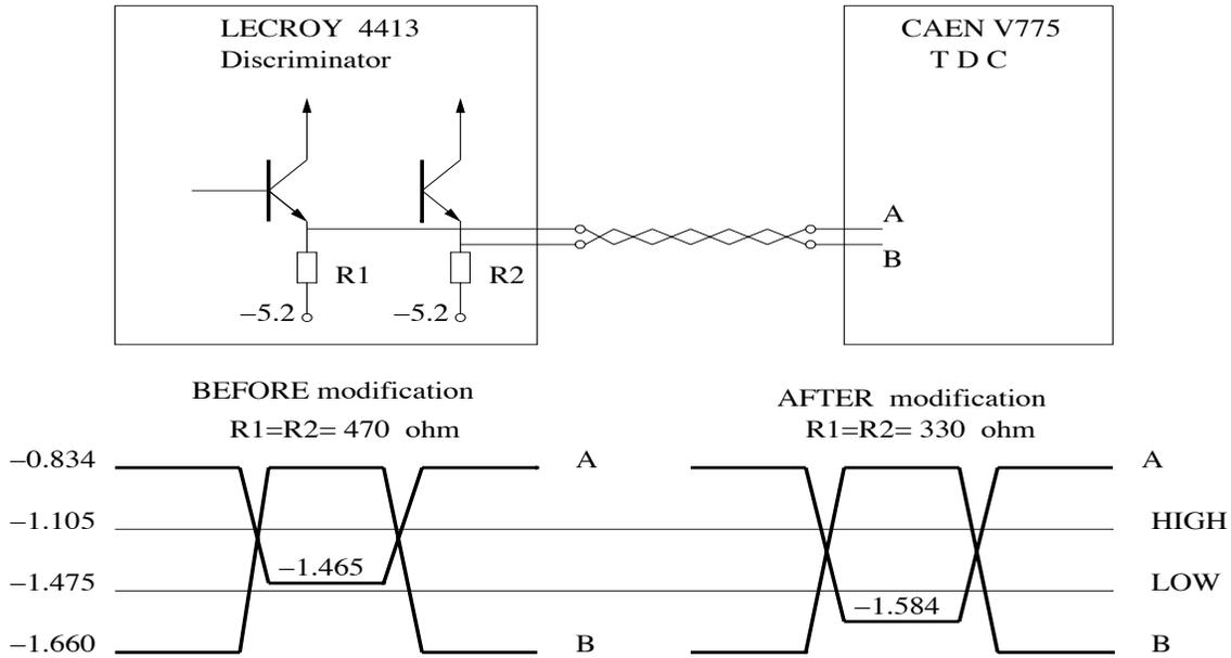
Figure 5: Discriminator signals before and after modification.
