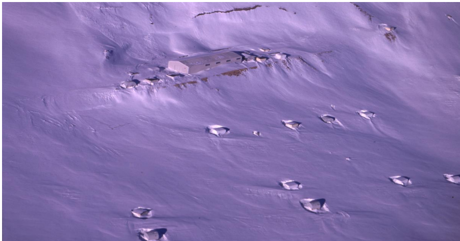
Figure 2: Aerial view of part of the EAS-TOP array during winter time. The e.m. modules are visible out of the snow; the muon detector is located inside the shed on top of the picture.
