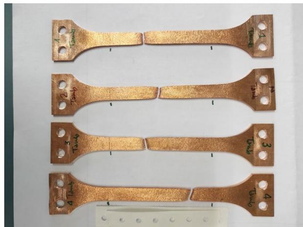
**Figure 4-23: Room temperature samples after rupture test.**
