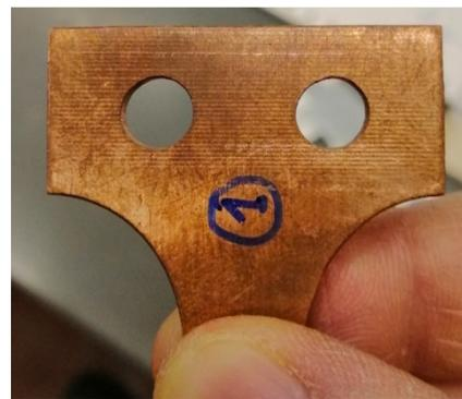
**Figure 4-5 Left: broken sample with indication of elongation. Right: detail of the head where the effect of the clamping can be seen. The tiny deformation of the holes is barely visible in this case**
