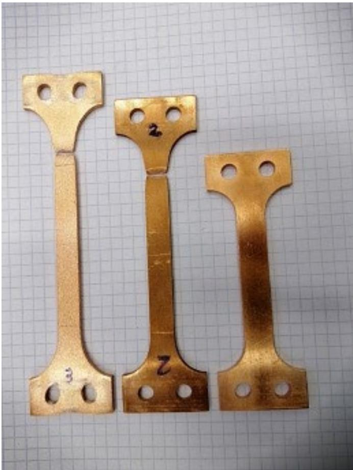
**Figure 4-12: Comparison among three samples: untested (right); tested without baking (center); tested after baking (left). It is evident how the baking affects the sample mechanical properties, with the material becoming much softer and losing elasticity. Plastic deformation sets in much earlier ( $R_{p0.2}$  ten times smaller), whereas the value of breakdown is around 82% that of the hardened material.**
