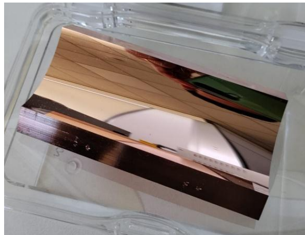
Figure 1: Left: CAD draft of the mount device used for the milling process of the copper sections. Right: Photo of one of the copper sections after the polishing and the diamond milling processes.
