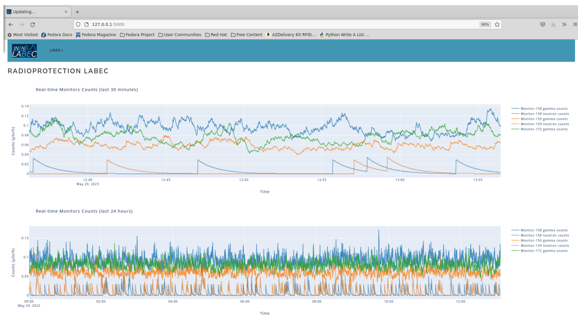
Figure 3: Screenshot of the page for real-time visualization of dose rates from all monitors for gamma rays and neutrons. Top: trending graph in the past 30 minutes; bottom: in the past 24 hours.
