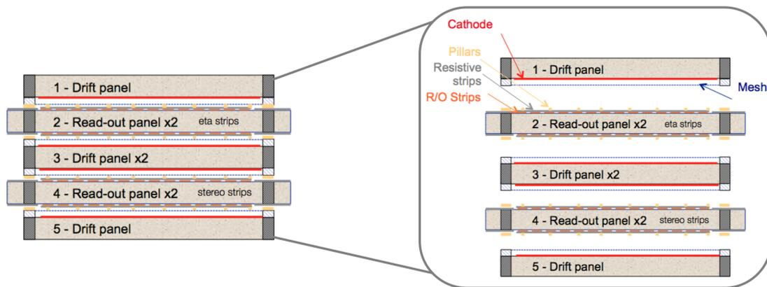
Figure 2: A schematic view of the five panels of a MM quadruplet.
