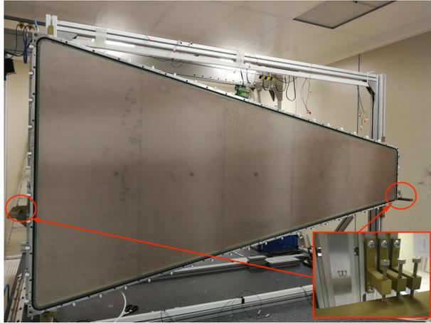
Figure 5: First External Drift in vertical position on the assembly tool.
