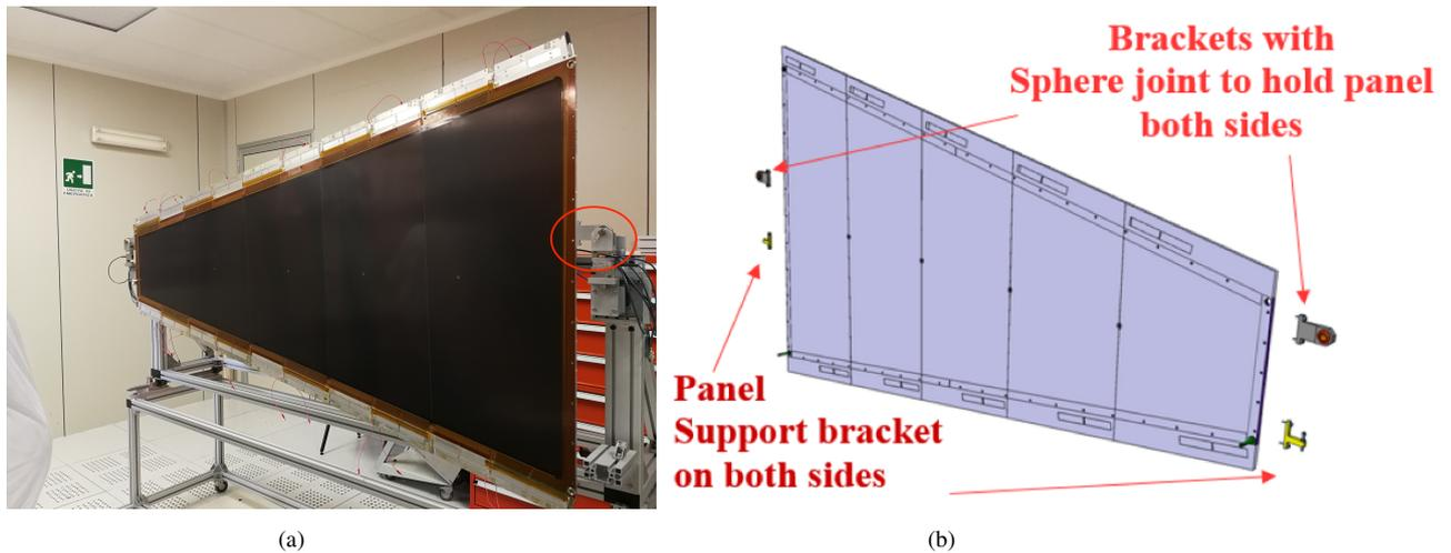
Figure 6: (a) Stereo Readout panel on the movable assembly tool. (b) Support bracket to hold the panel on the tool.
