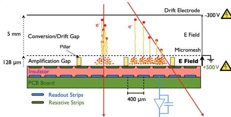
Figure 1: Schematic view of the micromegas detector and the principles of operation.
