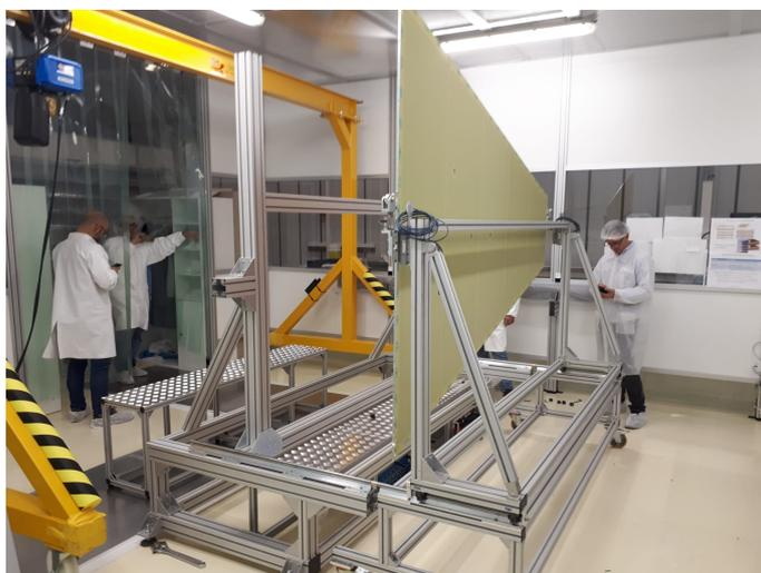
Figure 11: Copy of the LNF assembly system at Saclay production site.
