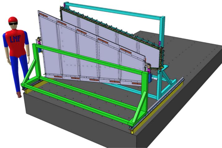
Figure 4: Picture of the assembly tool installed in the Clean Room at LNF.
