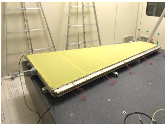
Figure 10: Assembled module on the granite table, ready to start the QA/QC tests.
