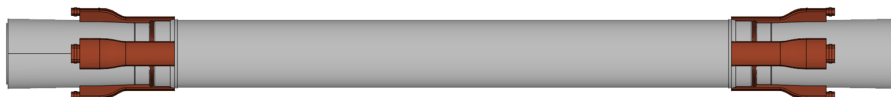
Figure 2: Central chamber in AlBeMet162 including cooling inlets and outlets for the Paraffin cooling circuit housed in a double layer, 180 mm long.
