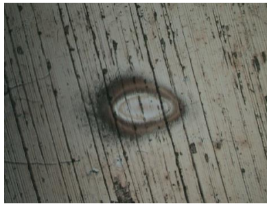
Figure 24: Large view optical image of the damage (the image is \sim 1 \times 1.5 mm).
