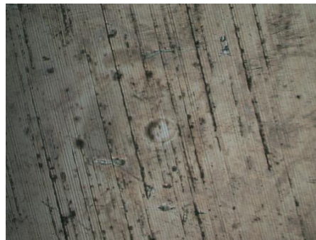
Figure 40: Large view optical image of the damage (the image is \sim 1 \times 1.5 mm).
