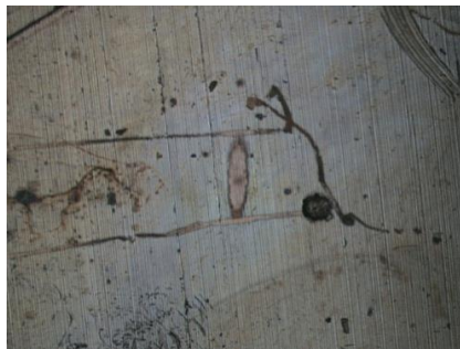
Figure 12 \text{MoO}_3 : Large view optical image of the damage (the image is \sim 1 \times 1.5 mm).
