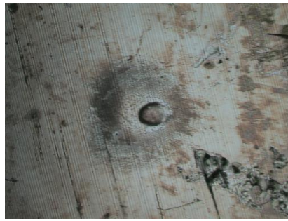
Figure 38: Large view optical image of the damage (the image is \sim 1 \times 1.5 mm).
