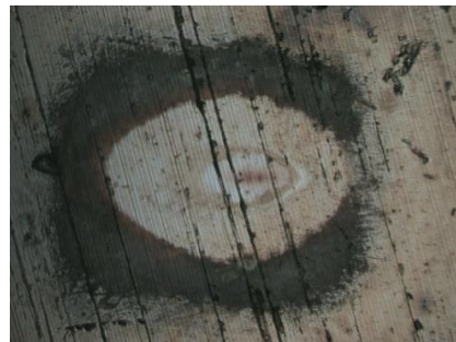
Figure 22: Large view optical image of the damage (the image is ~1x1.5 mm).
