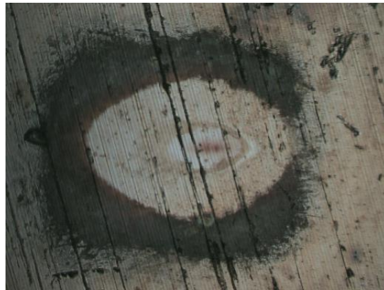
Figure 8: Large view optical image of the damaged area (the image is \sim 1 \times 1.5 mm).
