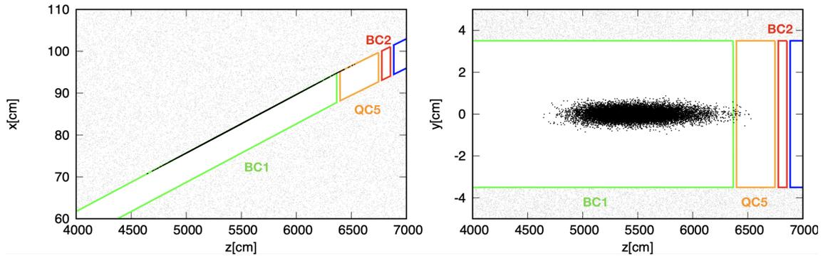
Figure 4: Map of the photons produced at the Z working point hitting on the beam pipe.
