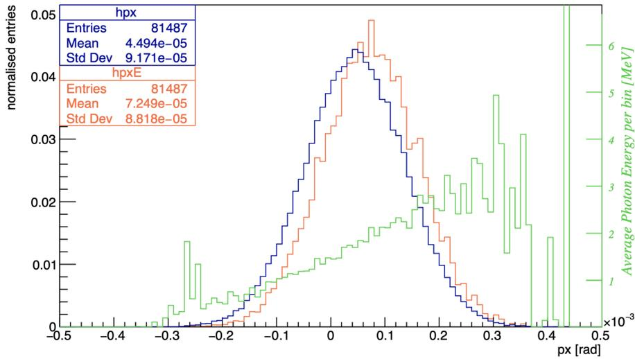
Figure 3: Comparison of the geometrical (blue) and weighted for the energy (red) horizontal angular distribution for the beamstrahlung photons emitted at the Z working point. In (green) the average photon energy per each angular bin.
