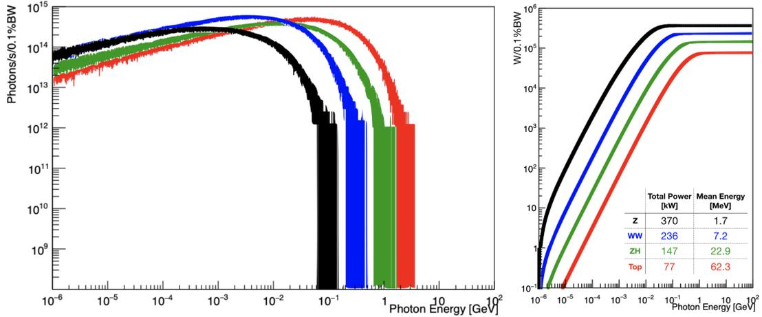
Figure 1: Left: flux of the beamstrahlung photons emitted at the four FCC-ee working points: 45.6 GeV (black), 80.0 GeV (blue) 120.0 GeV (green) and 182.5 GeV (red). Right: cumulative power distribution for the same working points.
