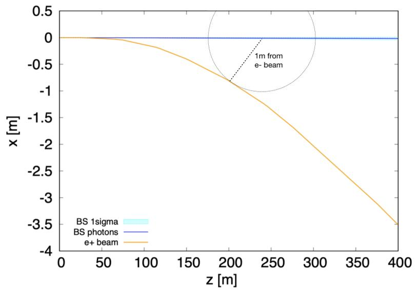
Figure 5: Top: sketch of the extraction line. Bottom: trajectories of the photon and electron beams.
