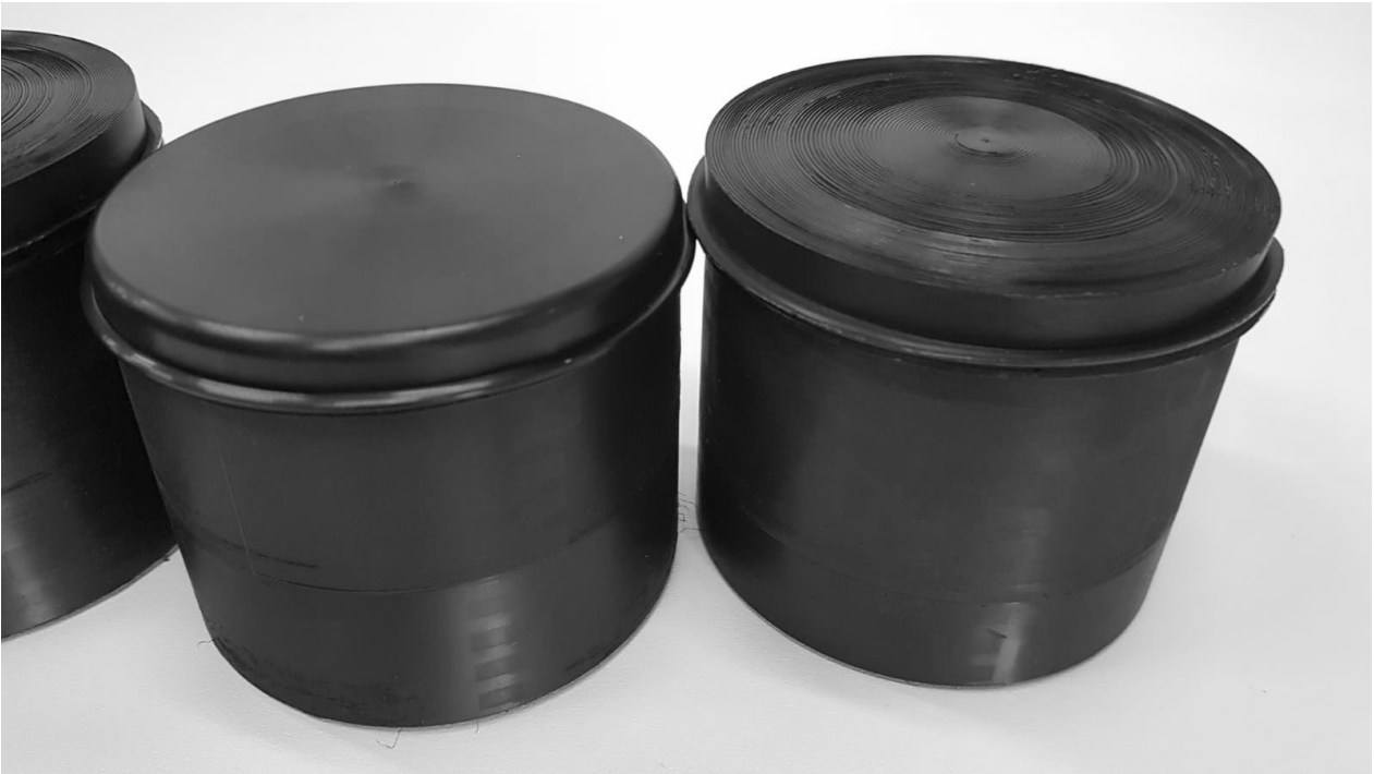
Fig.5: the spare BOBs after the sealing performed with the AWM. The contact region between the BOB and the cap are well visible in the upper part of the BOBs and look uniform
