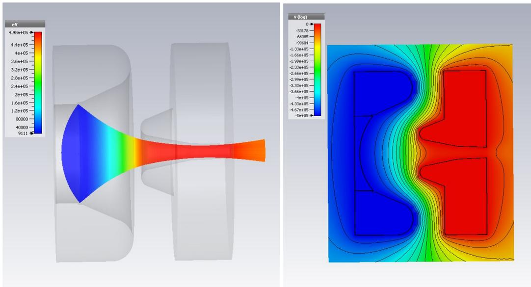
Figure 1: Preliminary electron gun design from CST. Beam trajectory (left) and Equipotential lines (right) are shown.
