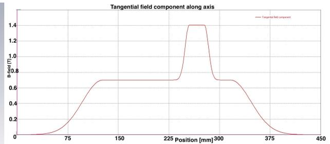
Figure 2: Beam trajectory along the propagation direction (left) and Axial magnetic field distribution (right) for two different models. Model 1 has a small peak of 14 KG model 2 has the same amplitude but a constant magnetic field about 30 mm at that manitude.
