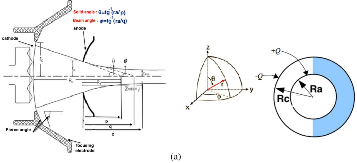
Figure 4: a) Schematic view of the Pierce-type gun geometry [11] b) Two concentric conducting spheres of inner and outer radii  $R_a$  and  $R_c$ , equivalent with the DC gun
