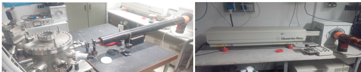
FIG. 1 - The PLD apparatus: the vacuum chamber (left) and the Nd:Yag laser (right) (Colour on line).
