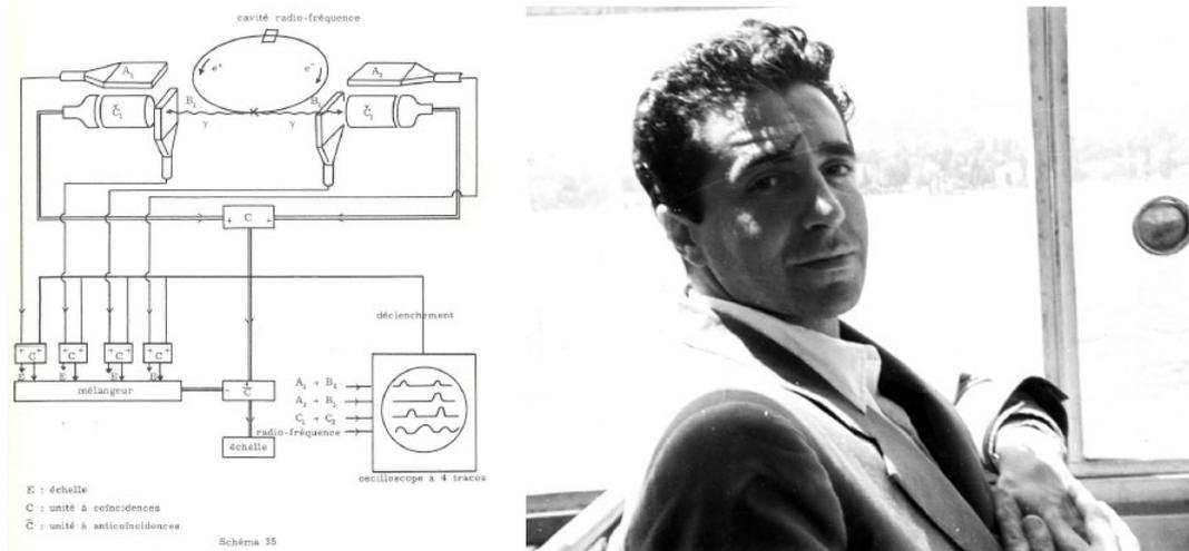
Figure 21: The logical scheme for measuring the process  $electron + positron \rightarrow 2\gamma$ , from Jacques Haïssinski’s thesis. The  $\gamma$  rays exiting AdA (center top) are depicted as two wavy lines labelled  $\gamma$ , to be detected by an assembly of electronics and detectors. The apparatus, was constructed by Giuseppe Di Giugno and Ruggero Querzoli, who is shown here in the right panel.
