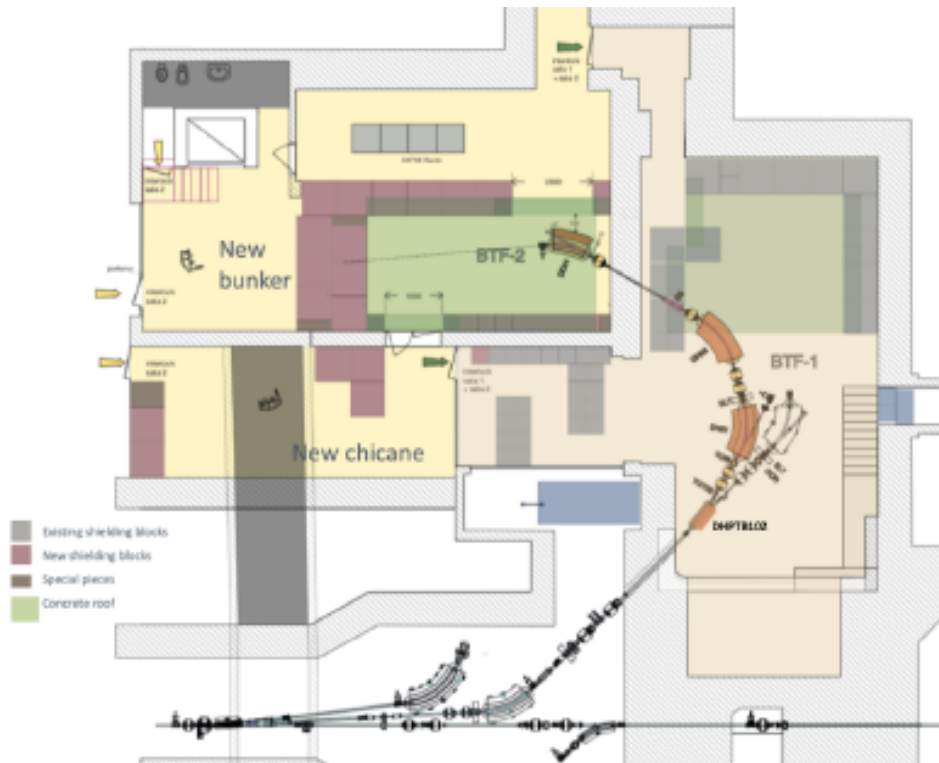
Figure 1 - New BTF and transfer line layout, showing the two new lines (BTF-1 and BTF-2) and the relative experimental halls.
