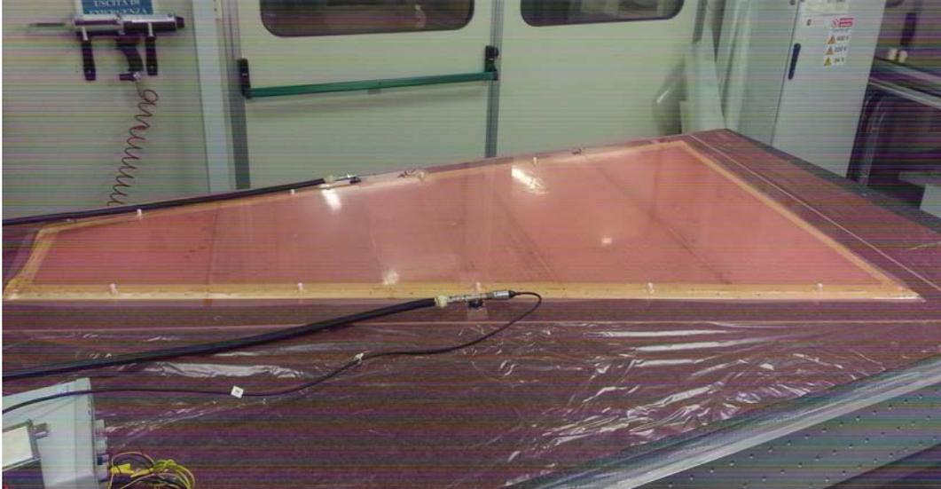
Figure 12: A drift panel during glue curing (vacuum bag technique) on the granite table.
