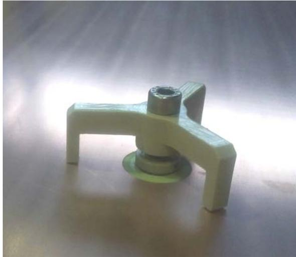
Figure 18: The plastic tripod to precisely position the interconnection drift spacers.
