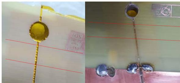
Figure 19: A junction between two PCBs in the o-ring region (red dashed lines) before (left) and after filling with Araldite 2011 (right).
