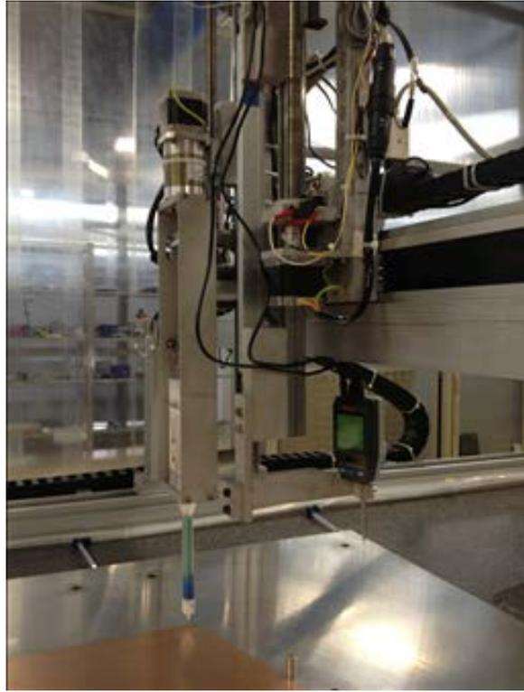
Figure 6: The height gauge and the glue dispenser.
