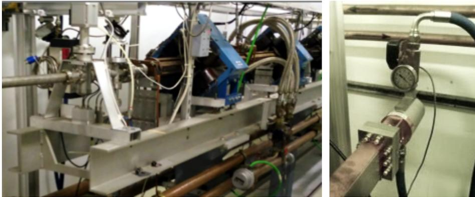
**Figure 3.10:** Left: the last SLAC type accelerating section at the end of the present LINAC is shown followed (from right to left) by the load, the diagnostics and vacuum pump; the two wrap-around quadrupoles (blue) and the cooling circuit pipes (bottom right) are also visible. Right: detail of the load with its cooling system.
