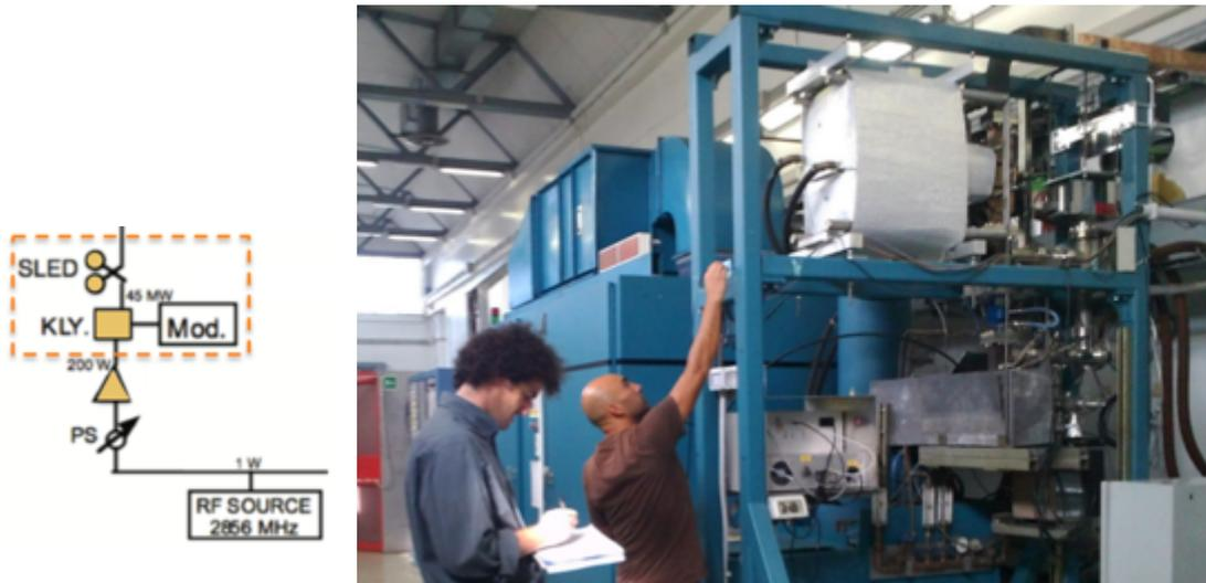
**Figure 3.1:** The RF power station (left, logical scheme; right, photograph): the 1 W RF from the 2856 MHz source, pre-amplified to 200 W by the RF driver, is amplified up to the maximum power by the klystron, fed by the modulator, and compressed by the SLED, prior to be distributed by the waveguide network to the accelerating sections.
