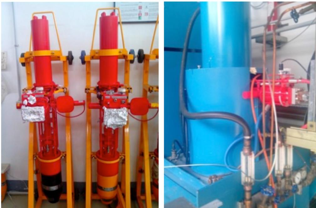
**Figure 3.5:** Left: two klystrons Thales TH2128C ready for installation; right: the klystron installed inside the cooling oil tank and surrounded by its focalizers.
