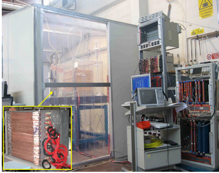
Figure 1: Schematic layout of the GGM system of the CMS RPC detector reproduced in the Frascati Laboratories.
