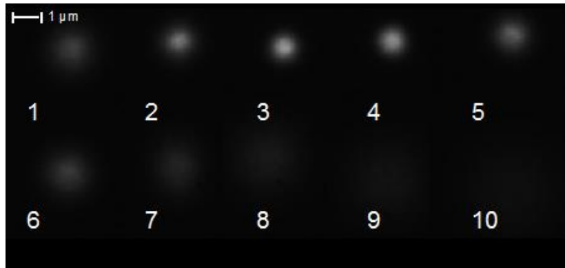
Figure 3: Set of images taken with the CCD at various distances: the picture 3 shows the better focused beam.
