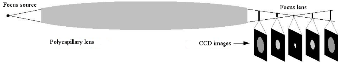
Figure 2: Scheme of a CCD camera image acquisition system, at various distances from the lens output.
