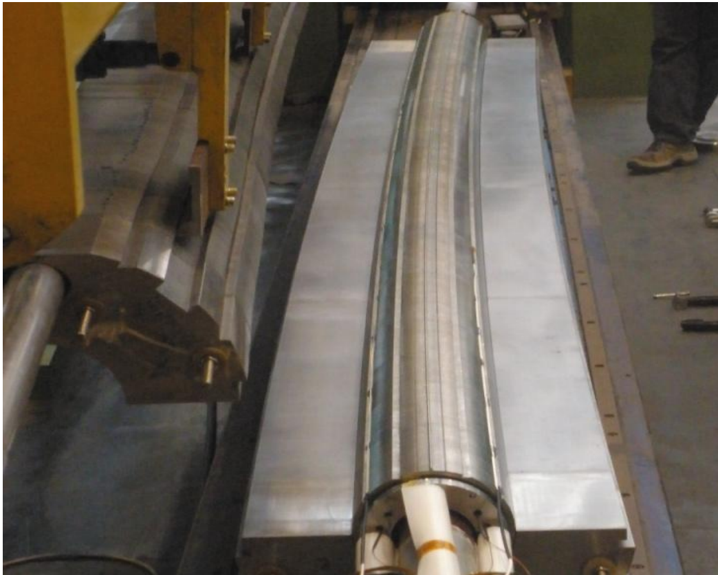
FIG.113: Lower half yoke hosting the collared coil. Both halves of the yoke are composed of four large blocks in silicon steel and two small blocks in stainless steel at the magnet ends.
